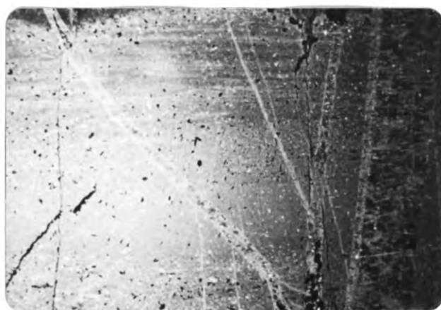
A. Displacement has occurred along the fractures, followed by quartz mineralization. The horse-tail fault and displacement of the northwest trending quartz filled fracture indicate the apparent direction of movement. The larger fracture contains quartz growing perpendicular to the fracture walls. Oxidation has taken place along bedding, and some of the fractures. Plain light, X3. Sample #2, slide B.
