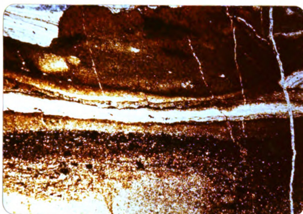
A. Structures associated with rock flowage. All of the fractures are younger than the features due to the period of flowage. Plain light, X3. Sample #6, slide A.
