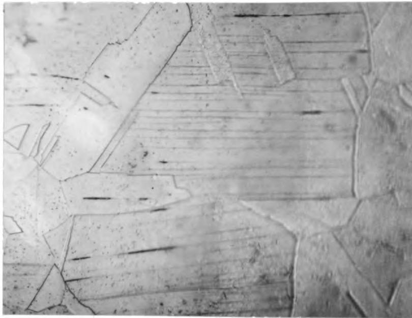
Figure 17. Taper section of peened bar after 2,560,000 cycles. Etched up slip bands in the center of the taper section. 500x.
