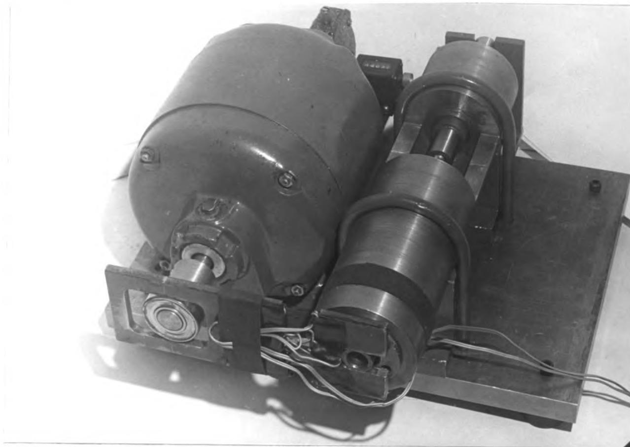
Figure 1. Constant strain amplitude fatigue machine, front view.
