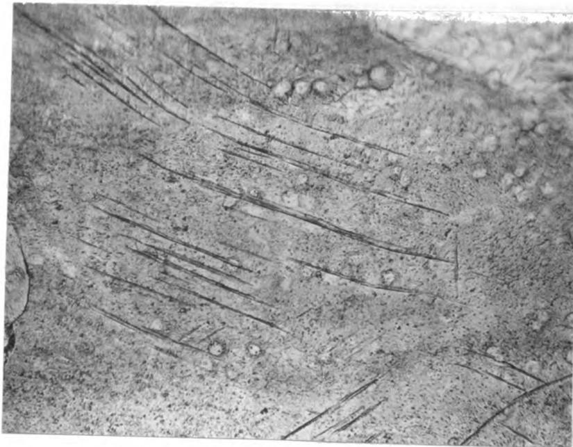
Figure 10. Taper section of peened bar after 5000 cycles. 500x.
