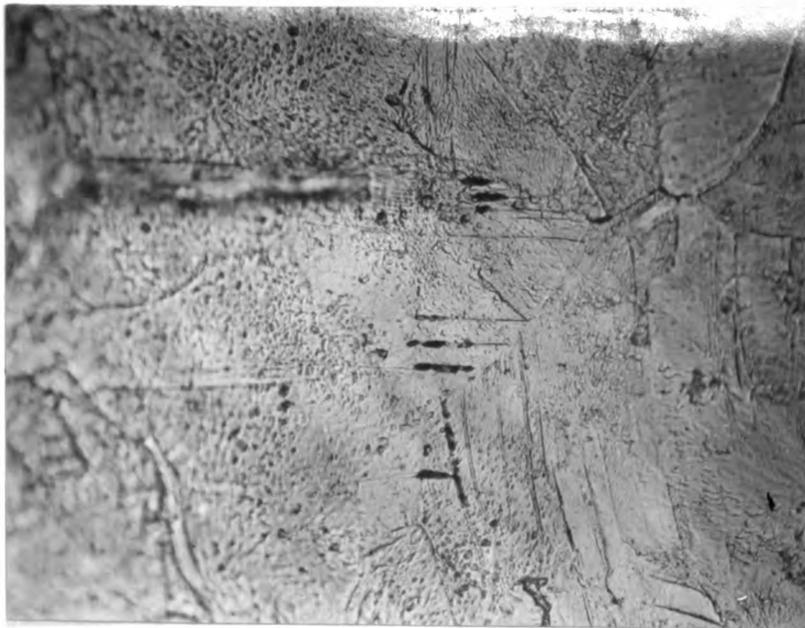
Figure 22. Taper section of peened bar after 10,240,000 cycles. Fissure and etched up slip at the surface. 500x.
