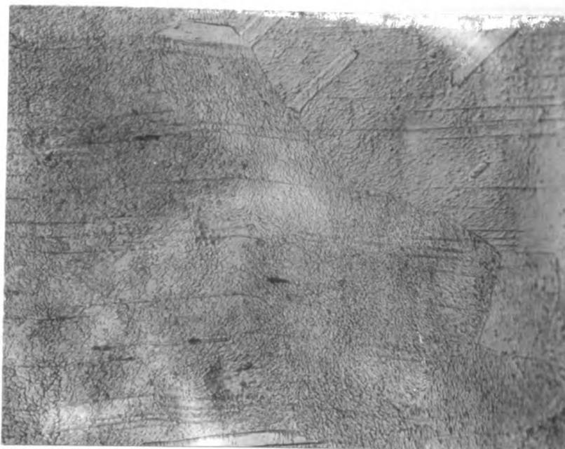
Figure 12. Taper section of peened bar after 640,000 cycles. Etched up slip bands near the center of the taper section. 500x.
