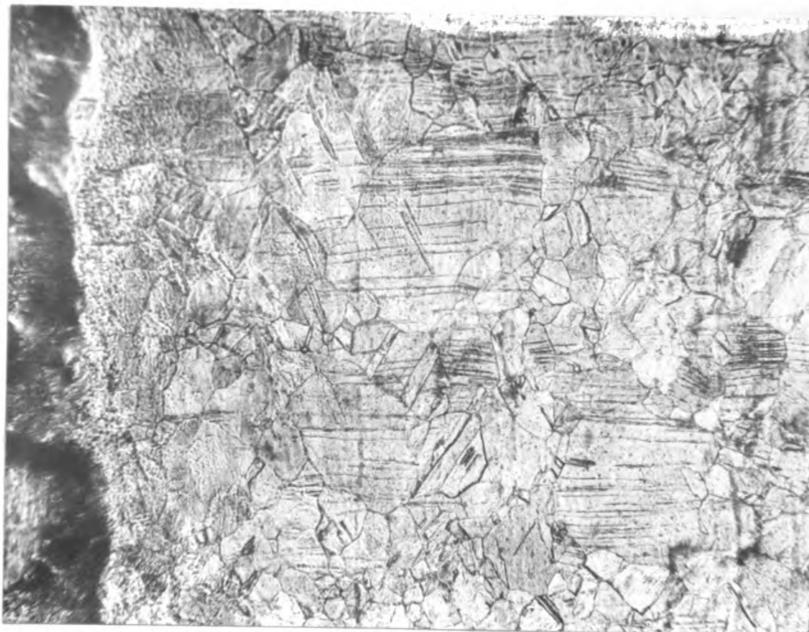
Figure 24. Taper section of peened bar after 10,240,000 cycles showing very little slip in the surface layer. 100x.
