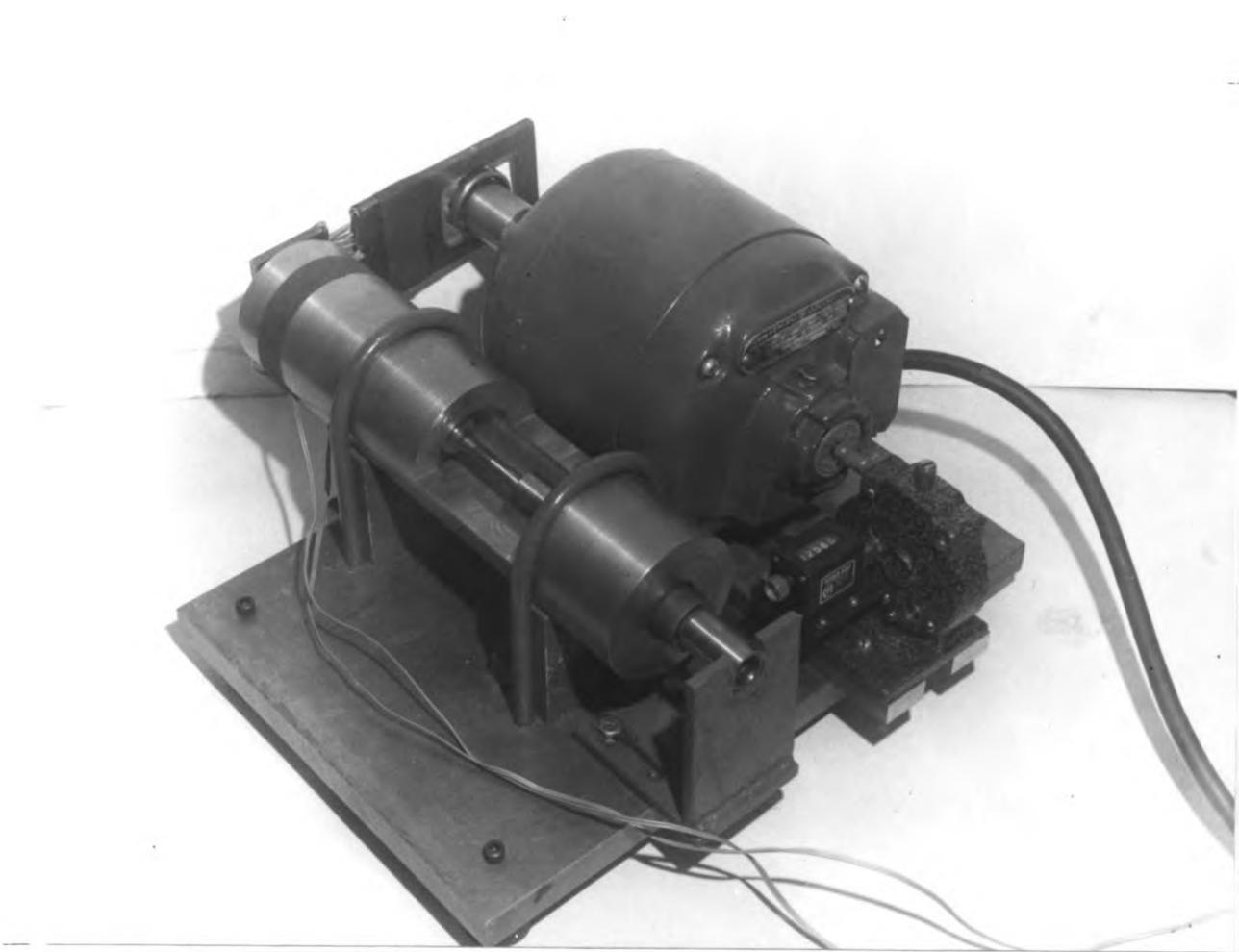
Figure 2. Constant strain amplitude fatigue machine, rear view.
