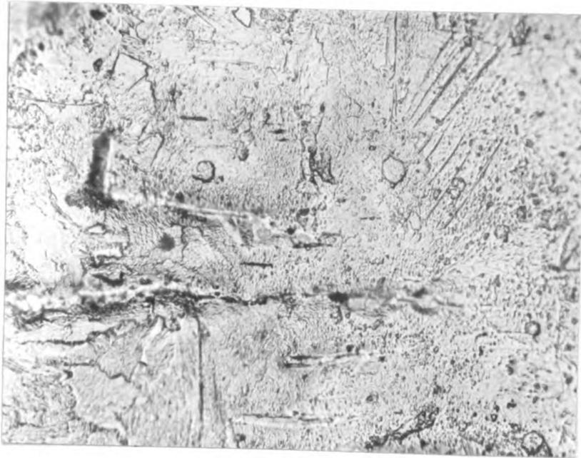
Figure 23. Taper section of peened bar after 10,240,000 cycles. Fissures and etched up slip markings near the surface. 500x.
