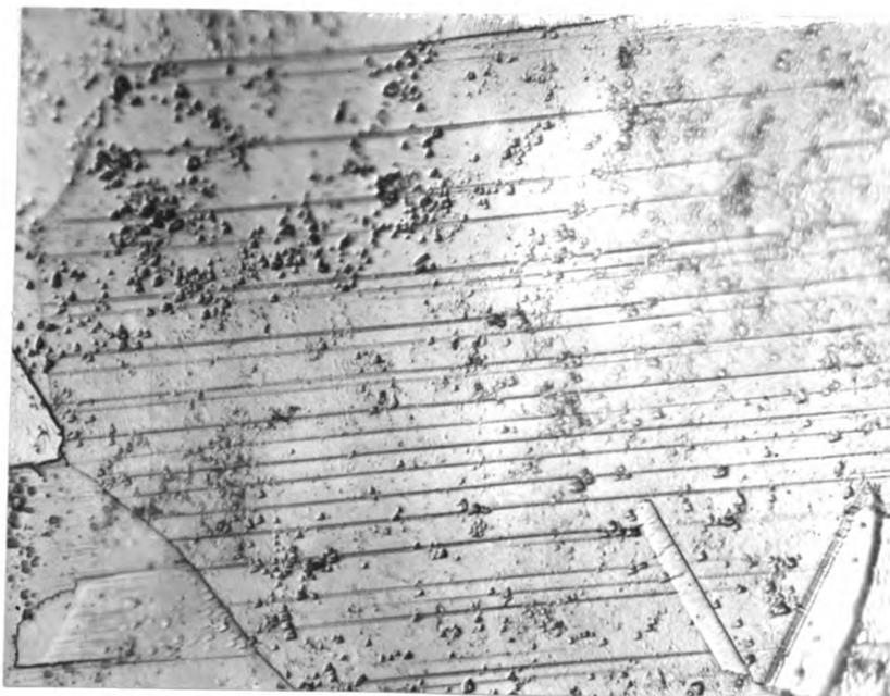
Figure 14. Taper section of polished bar after 640,000 cycles. Etched up slip bands at center of taper section. 500x.
