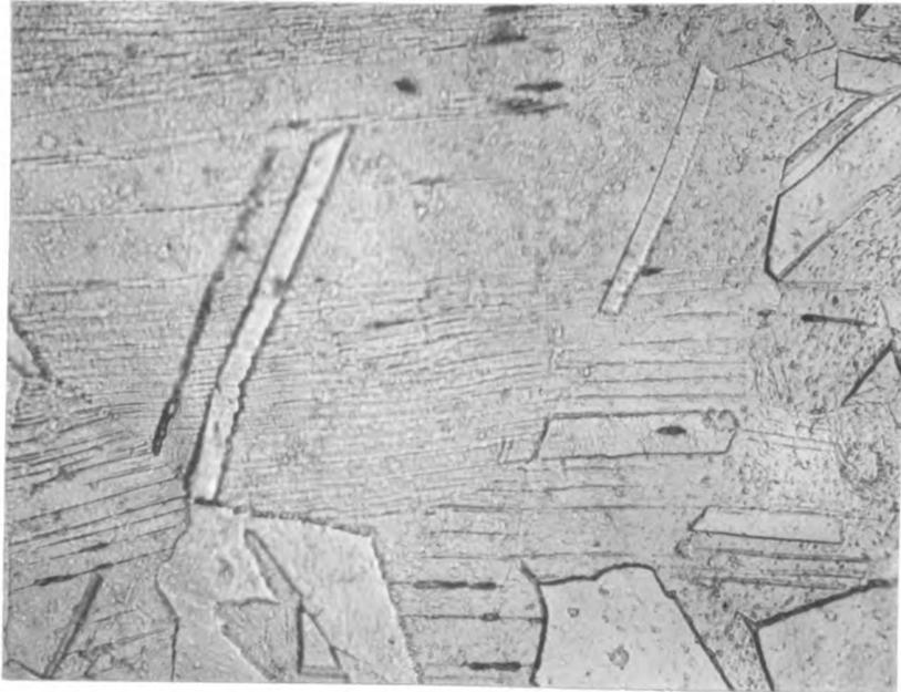
Figure 21. Taper section of peened bar after 10,240,000 cycles. Etched up slip bands near the center of the taper section. 500x.
