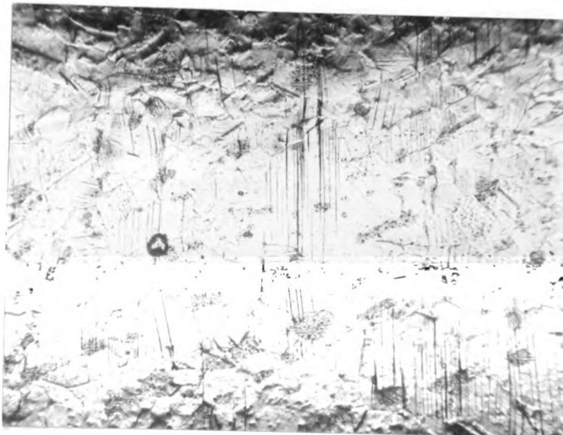
Figure 3. Surface of annealed and polished bar after 80,000 cycles. 100x.
