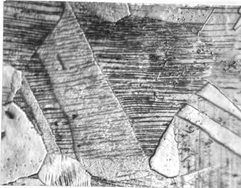
Figure 26. Taper section of peened bar after 20,000,000 cycles. Etched up slip bands in the center of the taper section. 500x.
