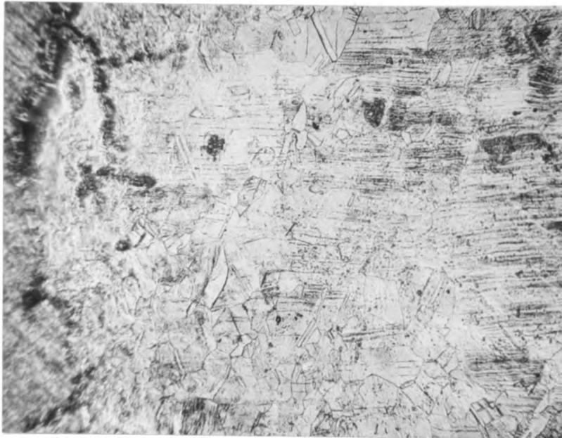
Figure 27. Taper section of peened bar after 20,000,000 cycles showing reduced number of slip bands at the surface. 100x.
