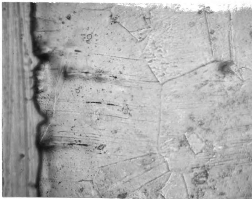
Figure 18. Taper section of polished bar after 2,560,000 cycles. Fissures and etched up slip bands at the surface. 500x.
