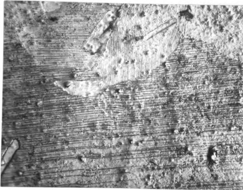
Figure 25. Taper section of polished bar after fracture at 10,920,000 cycles. Etched up slip bands near the fracture. 500x.
