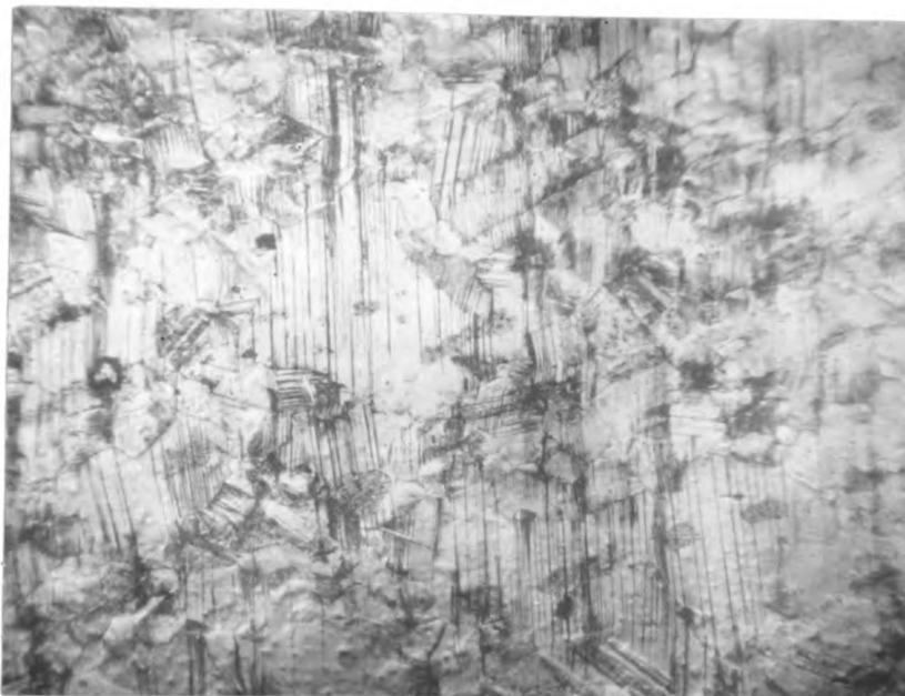
Figure 5. Surface of annealed and polished bar after 2,560,000 cycles. 100x.
