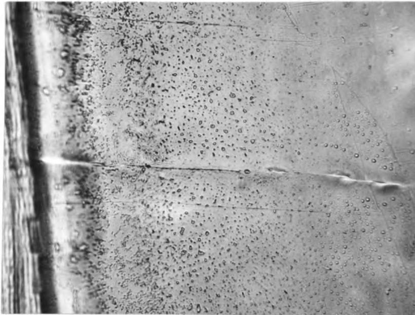
Figure 15. Taper section of polished bar after 640,000 cycles. Fissures visible at the surface before etching. 500x.
