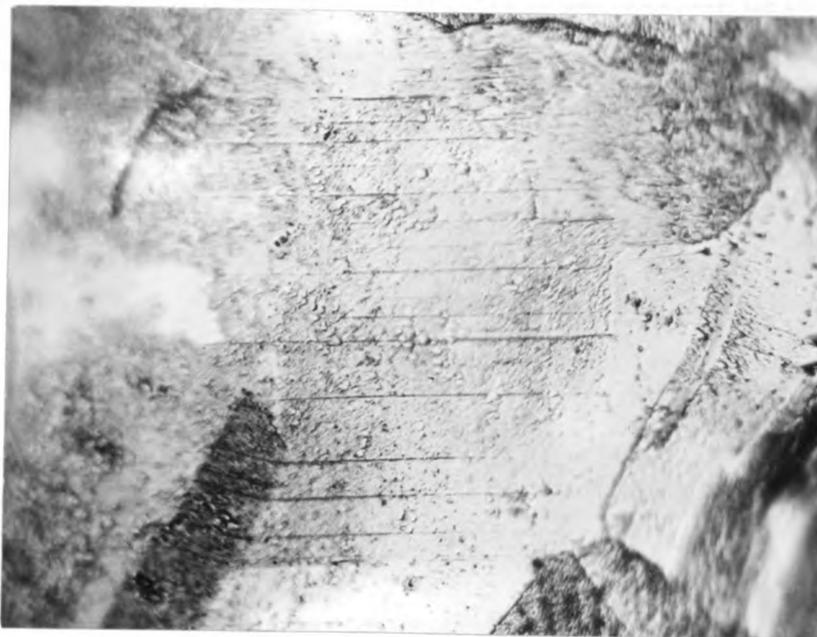
Figure 13. Taper section of polished bar after 640,000 cycles. Etched up slip bands near surface. 500x.
