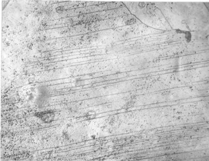
Figure 19. Taper section of polished bar after 2,560,000 cycles. Etched up slip bands near the center of the taper section.
