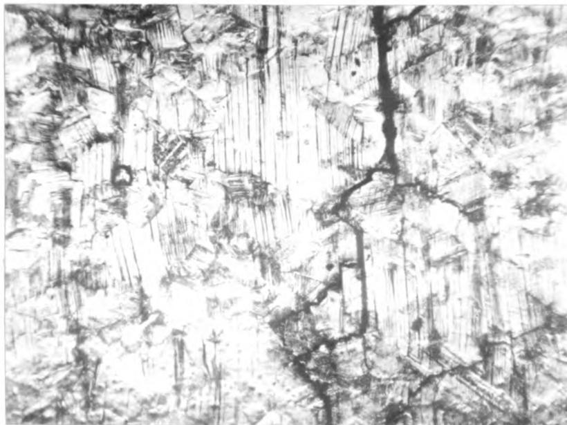
Figure 7. Surface of annealed and polished bar after 10,240,000 cycles. 100x.
