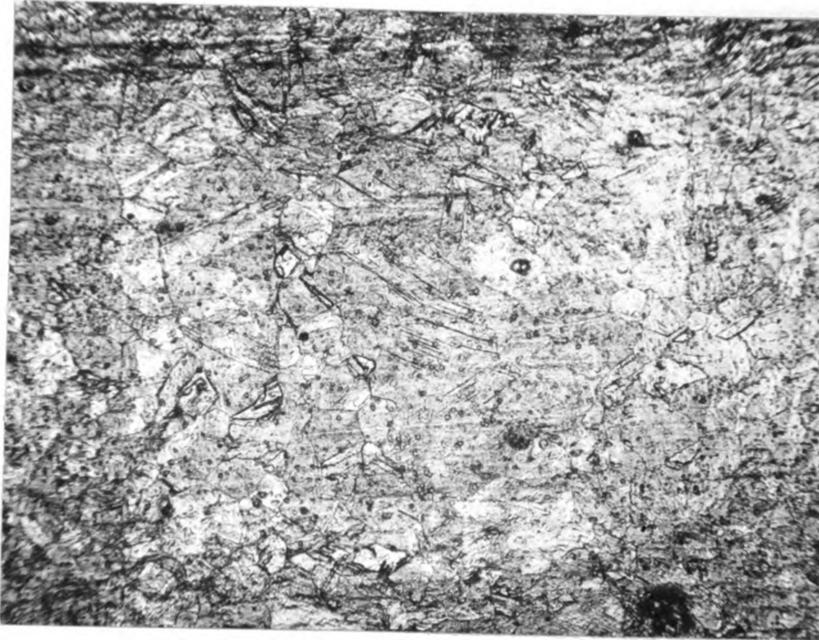
Figure 9. Taper section of peened bar after 5000 cycles. 100x.
