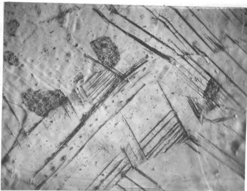
Figure 8. Surface of annealed and polished bar after 320,000 cycles. 500x. Oblique light.
