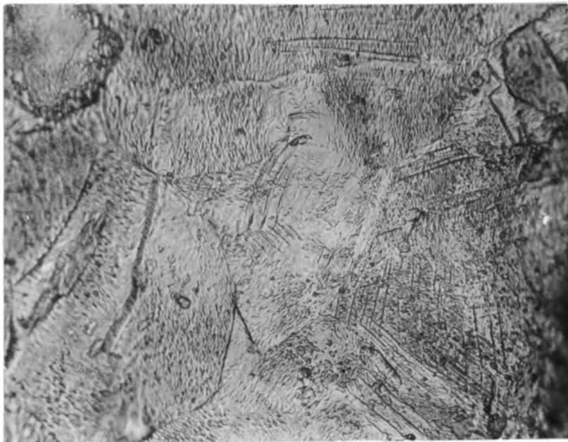
Figure 11. Taper section of peened bar after 640,000 cycles. Etched up markings near surface. 500x.
