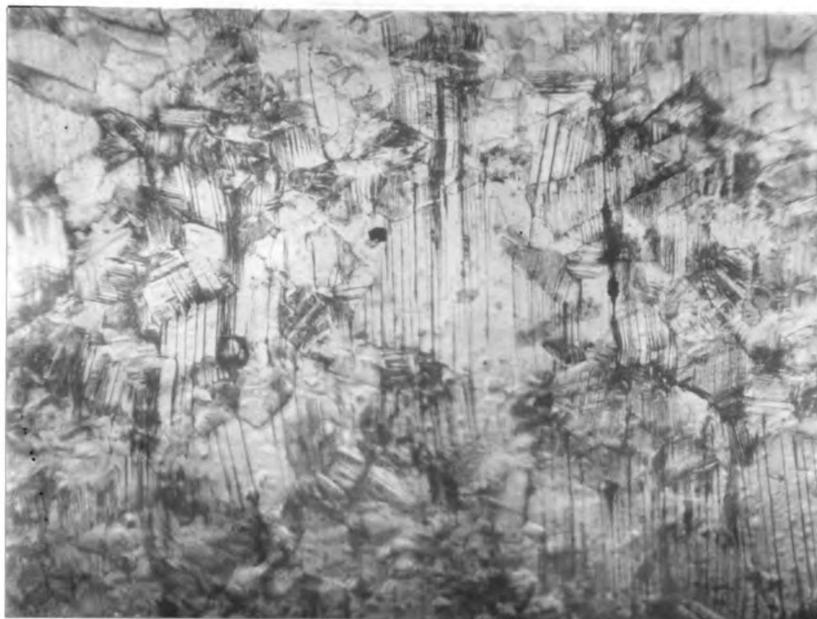
Figure 6. Surface of annealed and polished bar after 5,120,000 cycles. 100x.
