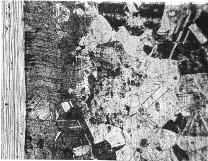
Figure 20. Taper section of polished bar after 2,560,000 cycles. Etched up slip bands at the surface. 100x.
