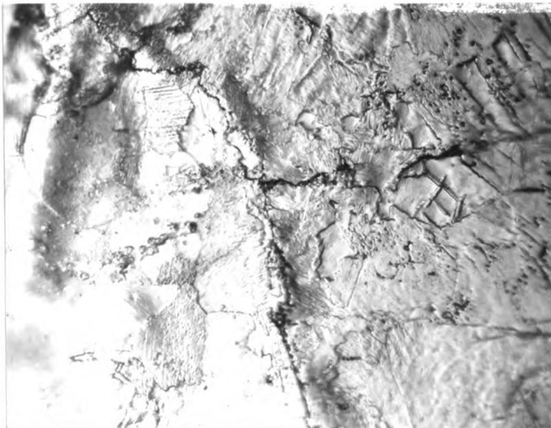
Figure 28. Intercrystalline crack visible in Figure 27 at 500x.
