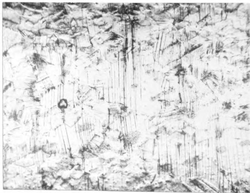
Figure 4. Surface of annealed and polished bar after 640,000 cycles. 100x.
