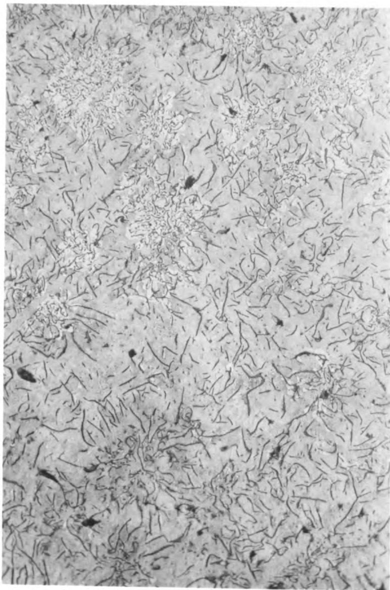
FIGURE 11 SAMPLE 2A3 SHOWING SURFACE GRAPHITE AND FERRITE Magnification--100x Etch-----2 % Nital Brinell-----4.18 mm. (209)
