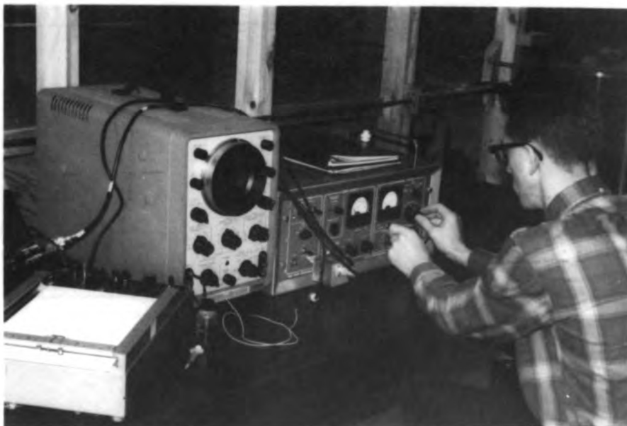
Figure 4.6. -- Apparatus used to measure and record air velocity fluctuations.
