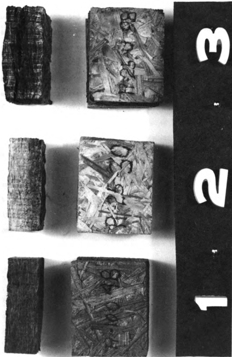
Figure 5. Degree of delamination in redwood particle boards. 1) 100% redwood, phenol-formaldehyde adhesive, 2) 25% redwood, phenol-formaldehyde adhesive, 3) 25% redwood, urea-formaldehyde adhesive.
