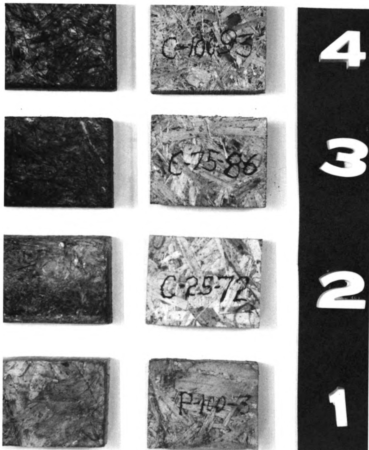
Figure 3. Appearance of decayed northern white cedar particle board; 1) 100% pine, 2) 25% cedar, 3) 75% cedar, and 4) 100% cedar. Boards at left illustrate surface in contact with feeder strips, upper face shown at right.
