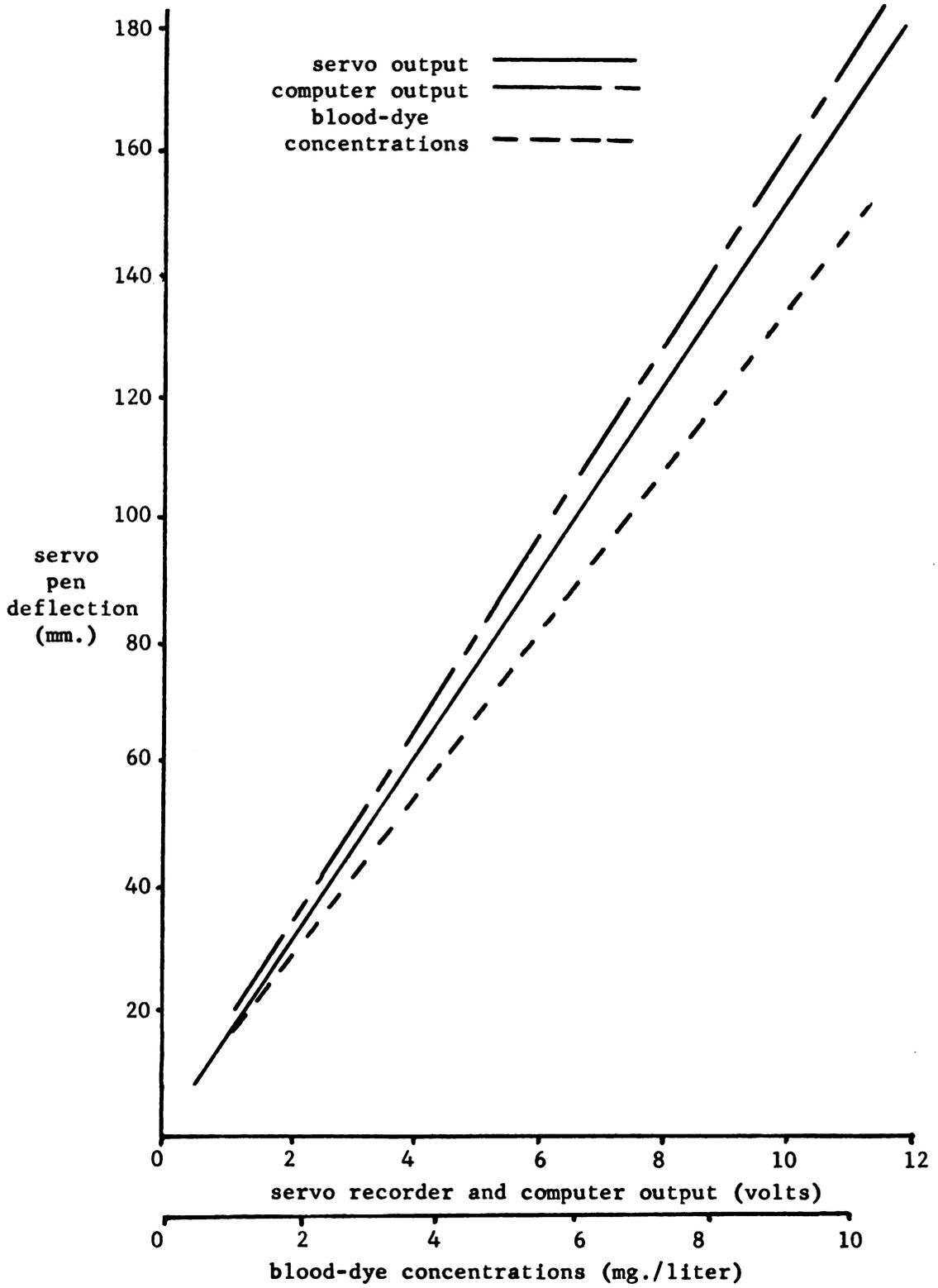
Fig. 3 Graph of Servo Pen Deflection vs. Servo Output Voltage, Computer Output Voltage, and Varying Blood-Dye Concentrations
