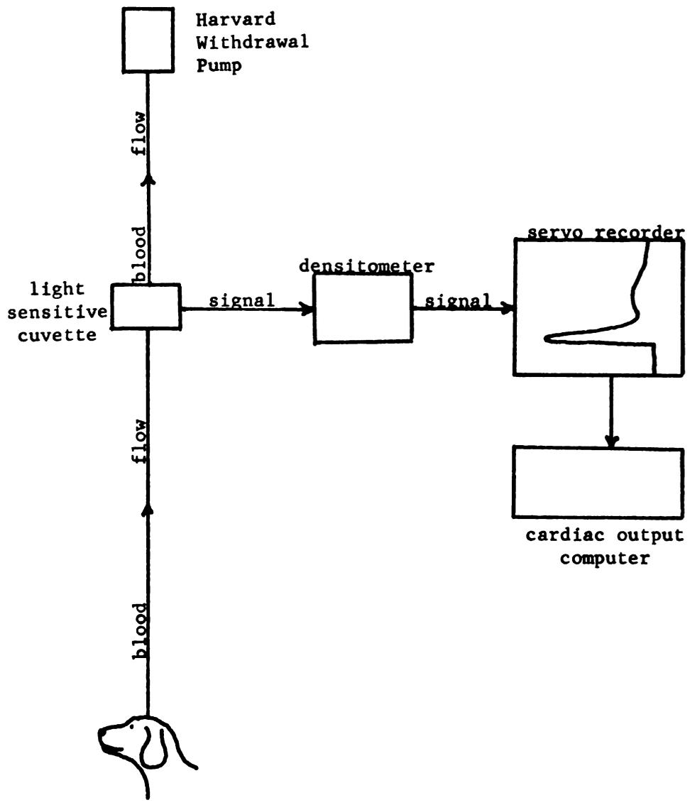
Fig. 2 System for Recording Cardiac Output
