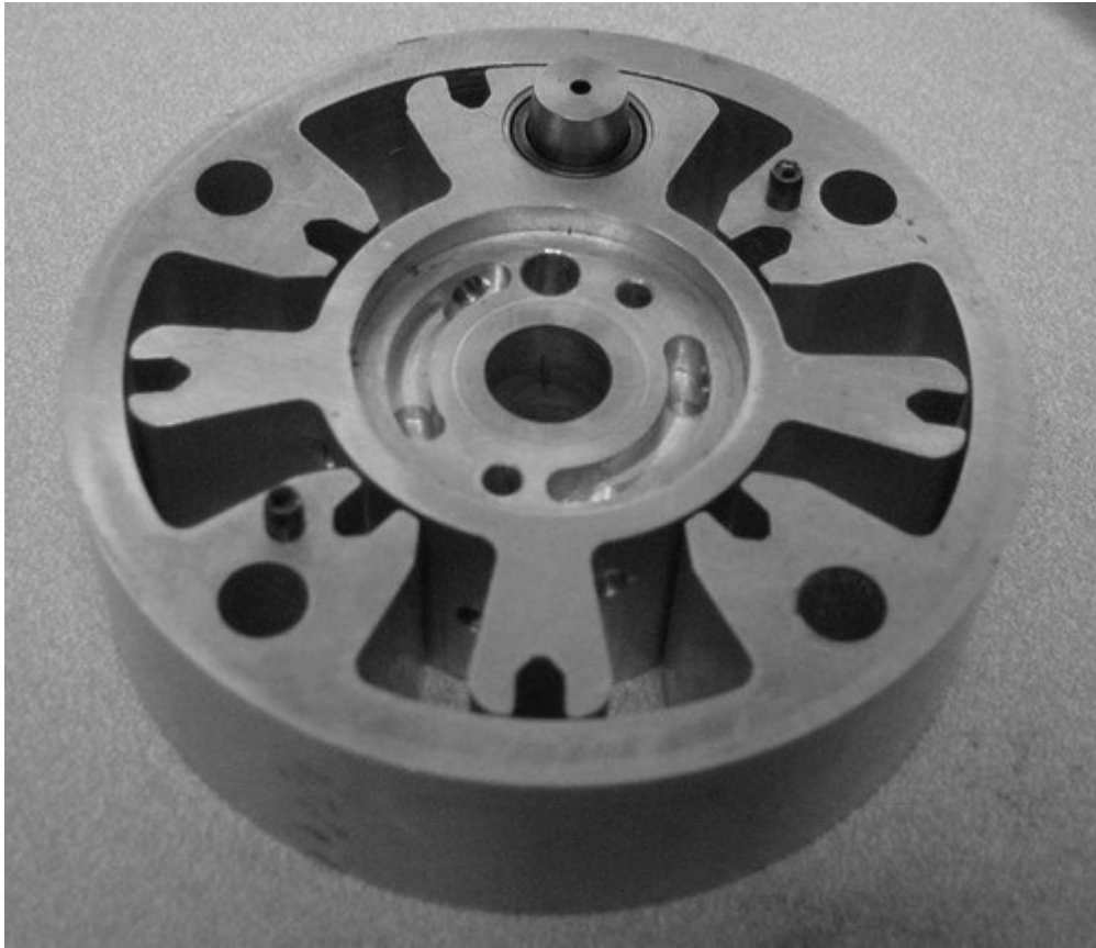
Figure 3-10. Vane type cam phase hydraulic pulley
