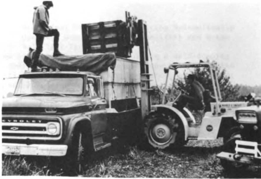
Figure 5. Experimental Mechanical Harvesting System IV in Operation in Southwestern Michigan Utilizing the 8-ton Bulk Tank Trucks and Rotary Head Field Forklift to Empty Pallet Containers.
