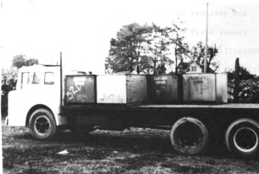
Figure 4. Existing Mechanical Grape Harvesting System III in Operation in Southwestern Michigan Utilizing Cherry Tank Containers Instead of Plastic Lined Pallet Containers to Transport Harvested Grapes to Processing Plant.
