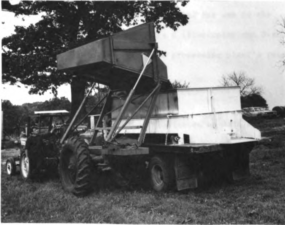
Figure 7. Self-dumping 3-ton Vineyard Totelift Discharging into an 8-ton Capacity Bulk Tank Truck (System V).
