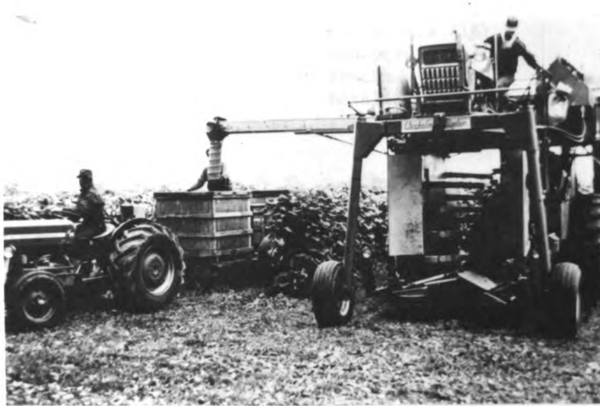
Figure 3. Existing Mechanical Grape Harvesting System II in Operation in Southwestern Michigan Utilizing Plastic Lined Pallet Containers to Transport Harvested Grapes to Processing Plants.
