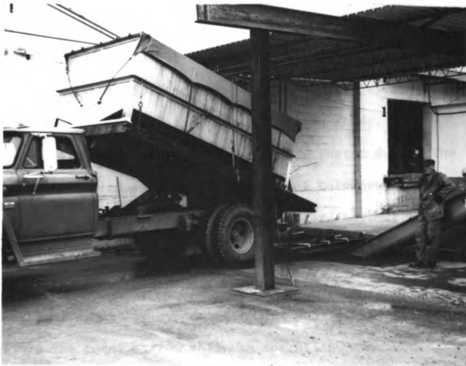
Figure 7. Self-dumping 3-ton Vineyard Totelift Discharging into an 8-ton Capacity Bulk Tank Truck (System V).
