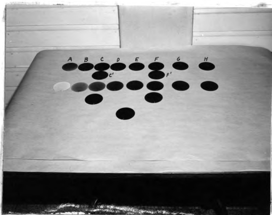
Figure 10 Blackened collection disks showing results of charged and uncharged dust as a function of distance
