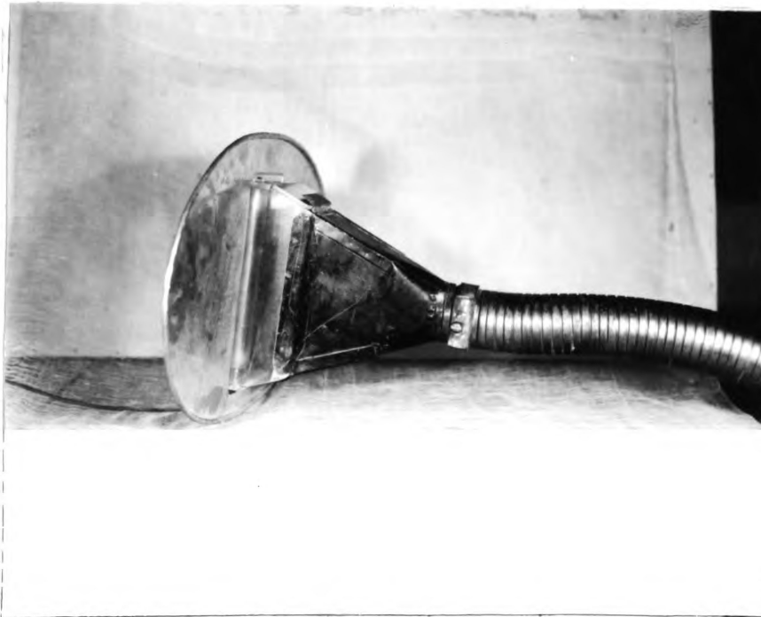
Figure 5 Manner of attachment of electric charging head to dust distributor tubes
