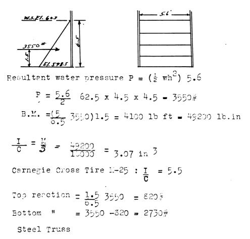
This truss will be rather unusual in that it must support its own weight in a horizontal position, a dead load of a temporary foot bridge, a live load and impact, and the horizontal panel point load, the loading which makes the truss necessary.
