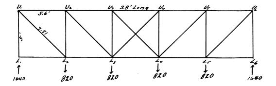
Length of diagonal = Influence line for shear in panel 1-2 Influence line for shear in panel 2-3 ÷ J. Influence line for shear in panel 3-4 ÷ 5 6 Full load stresses (horizontal) (by index method) Lember Index Stress Factor Stress -1837 -1640 5,5,6,0,0,5,6,5,6 V, -V2 -2460 -2755  $V_{1} - V_{J}$ -2460 -2755 V, -V, -2460 -2755 V. -V. -1640 -1837  $V_{f} - V_{c}$ 0  $L_i - L_i$ 0 ±1640 ±1837  $L_{1} - L_{2}$ **1**2460 **1**2755 L, -L,  $L_y - L_s$ **1**1640 11837  $L_{f} - L_{L}$ 0 0 -1640
