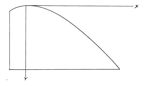
Representative coordinates of curve for unit head and upstream face vertical
