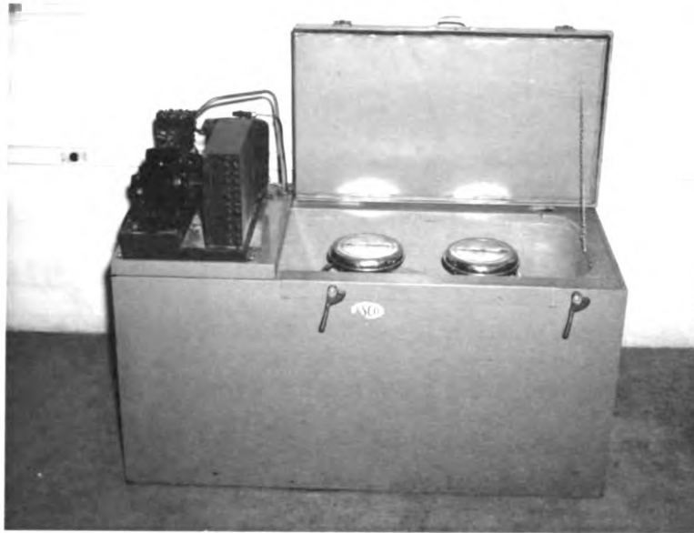
Figure 7. Standard Milk Cooler For Farm Milk Cooling.
