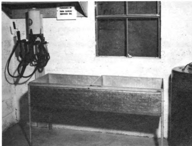
Figure 10. Double Wash Vats For Washing And Sterilizing Milk Handling Utensils.
