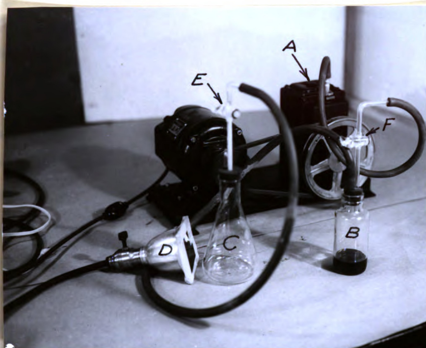
Figure 15. The vapor state fluorescence detection apparatus is shown above. The vacuum pump (A) was connected to the oil sample bottle (B) through suction tubing and the stopcock (F). The oil sample bottle was connected to the fluorescence detection flask (C) through suction tubing and the stopcock (E). The filtered lamp (D) was used as a source of ultra-violet radiation.
