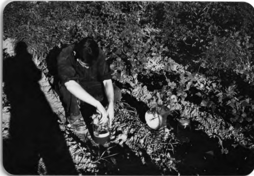
Figure 12. The washing procedure was carried out as illustrated above. Samples of a definite size were washed by immersion to remove the dust deposit, a measured quantity of washing solution being used. The red color of the washing is evident.
