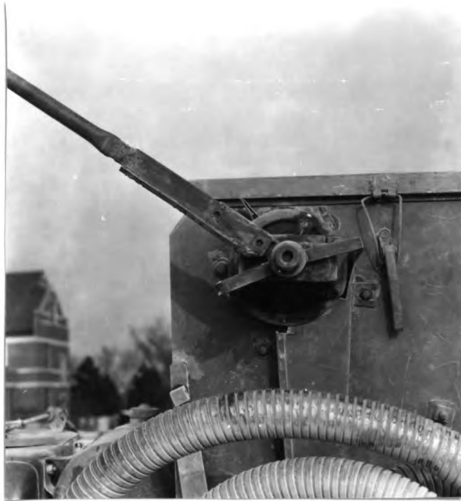
Figure 9. The above view shows the duster feed-cutoff mounted on the metering drum, at the rear of the duster hopper. An operator, standing on a platform on the rear of the machine could control the dust flow and charging apparatus as the duster passed from plot to plot.
