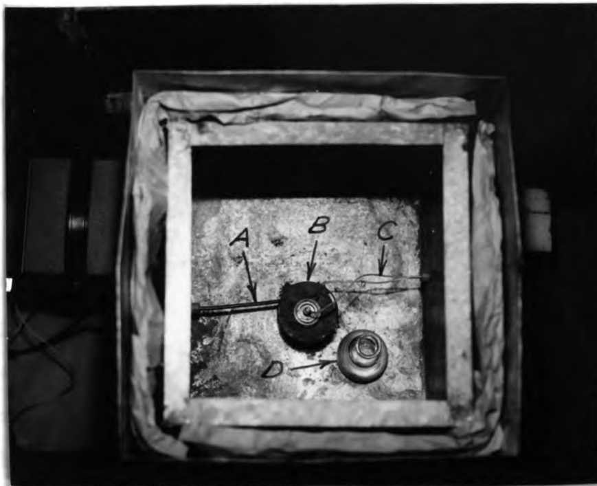
Figure A-4. The above illustration shows the interior of the resistometer chamber. The high-voltage in put cable (A) leads to the electrode cup containing the dust sample (B), and the wires (C) lead from the ground electrode on the dust surface. The flask (D) contained water for the constant wet-bulb thermometer.
