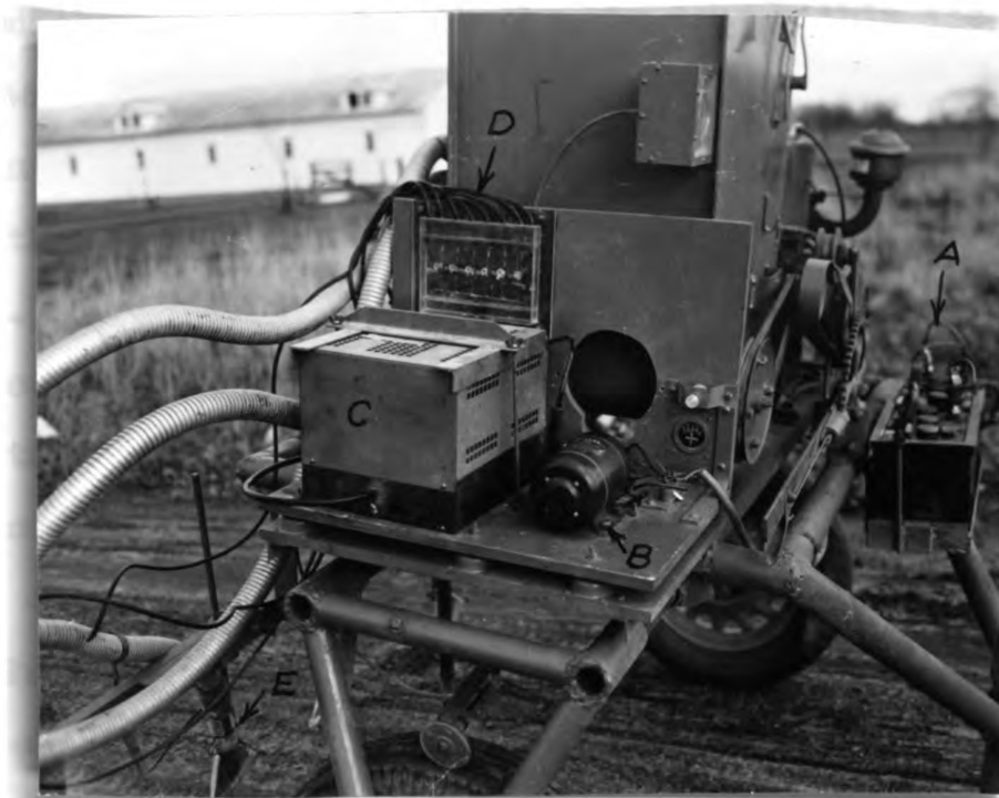
Figure 3. An experimental field duster equipped for electrostatic charging is shown above. Low voltage direct current supply from the storage batteries (A), is "converted" to a direct current supply of about 300 volts by the dynamotor (motor-generator) (B). This input is fed into the electronic oscillator voltage-tripler (C), which produces the required direct current charging potential of about 12,000 to 15,000 volts. The high voltage output is delivered to the charging nozzles (E) through high voltage cables (D).
