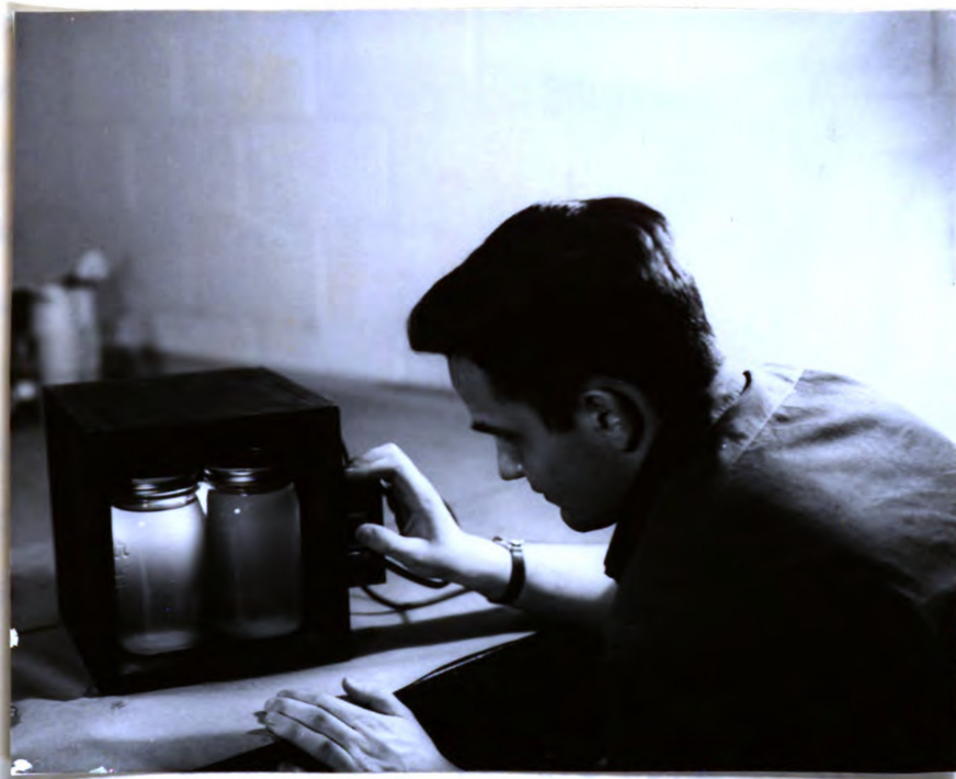
Figure 14. The final evaluation of deposition was performed with the aid of a standard light source. The samples were visually compared with standard color solutions, thereby enabling estimation of sample concentrations.
