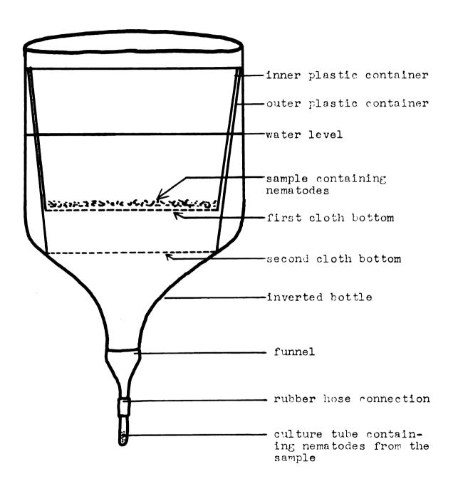
Diagrammatic sketch of inverted bottle used to collect nematodes from soil and plant samples.
