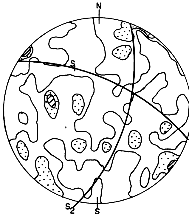
Fig. 8. Sample 13, 400 quartz c-axes. Contours 3-2-1%. S_1 is the bedding plane. S_2 is a joint surface.
