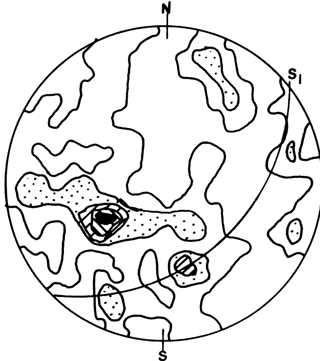
Fig. 9. Sample 11, 100 quartz c-axes from quartz vein. Contours 9-7-5-3-1 %. S_1 is the surface of the vein walls.
