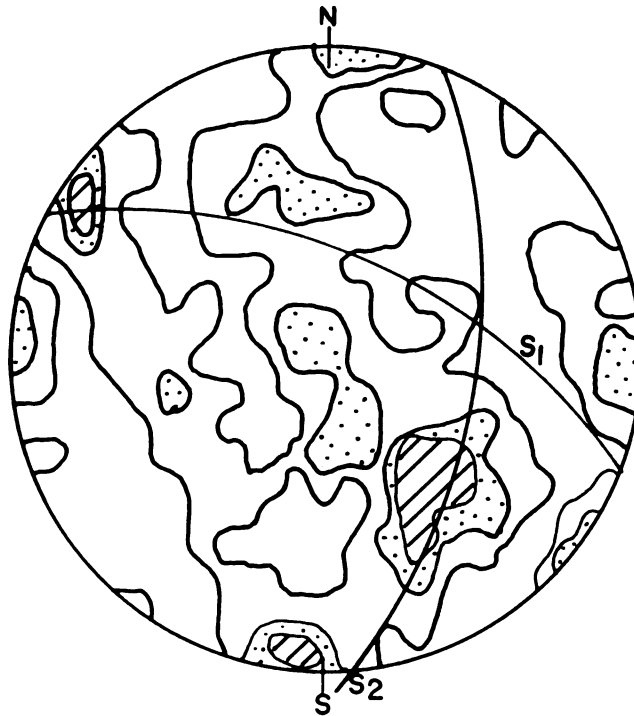
Fig. 7. Sample 12, 400 quartz c-axes. Contours 3-2-1%. S_1 is the bedding plane. S_2 is a joint surface.
