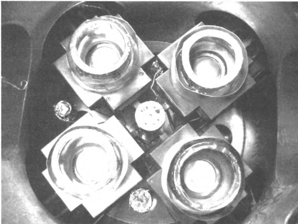
Figure 5.3: Top view of 4 main triode sputter sources as well as two smaller magnetron sources.
