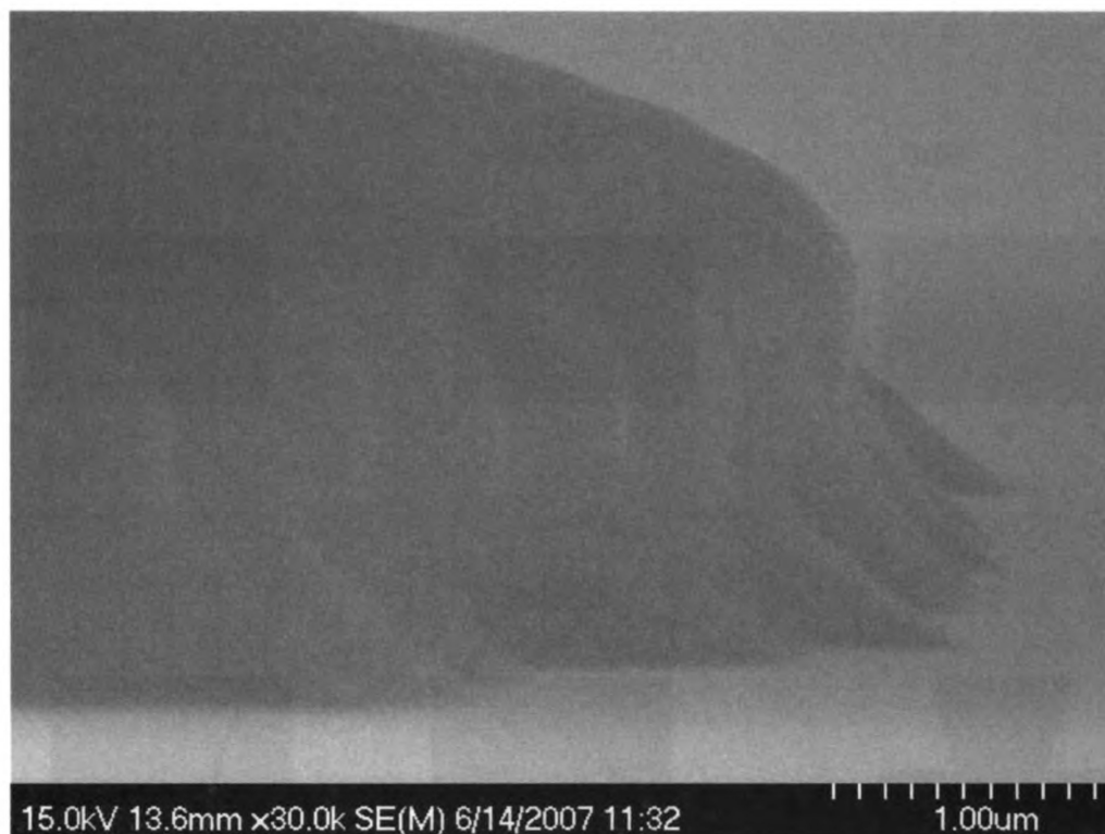
Figure 5.8: Sample over baked ( 115^{\circ}\text{C} ) after exposure.
