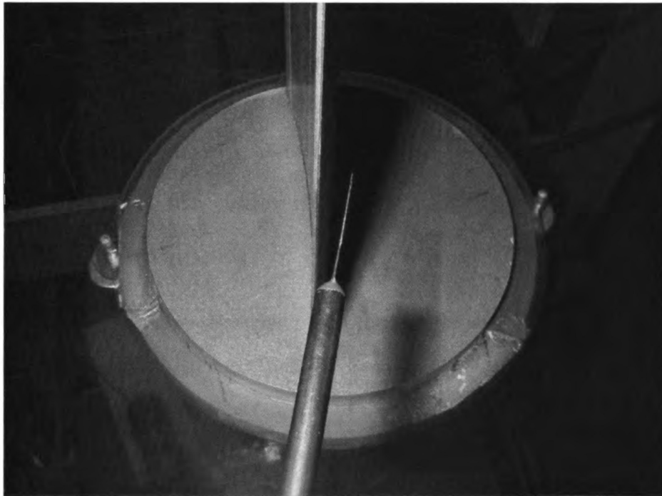
Figure 5.31: Top view of HW probe traversing the near wake region.
