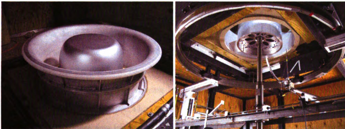
Figure 3.9: RCDB final design installed (left - upstream view; right - downstream view).
