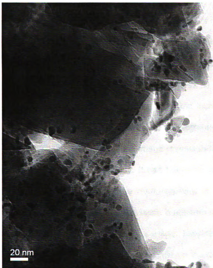
Figure 4.15. Bright field TEM image of Pt particles (dark spots) decorating the surface of oxygen-terminated diamond powder. The loading was 18 % Pt/C.
