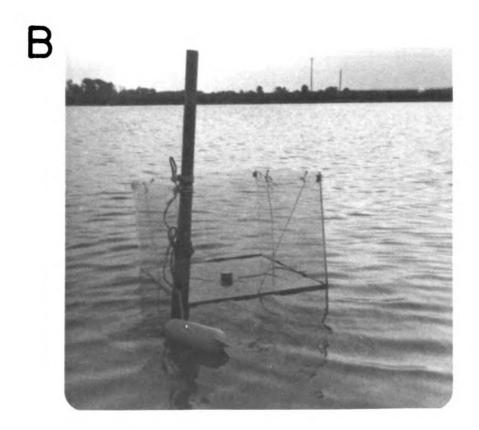
surface gas exchanges was eliminated by covering the enclosed water with adjustable plexiglass lids. The particular technique was based on the light-dark bottle concept of Gaarder and Gran (1927). By measuring oxygen changes between dawn and dusk, it was possible to estimate net primary production (NP); the differences between oxygen concentrations at dusk and the following dawn were taken as estimates of respiration (R).
