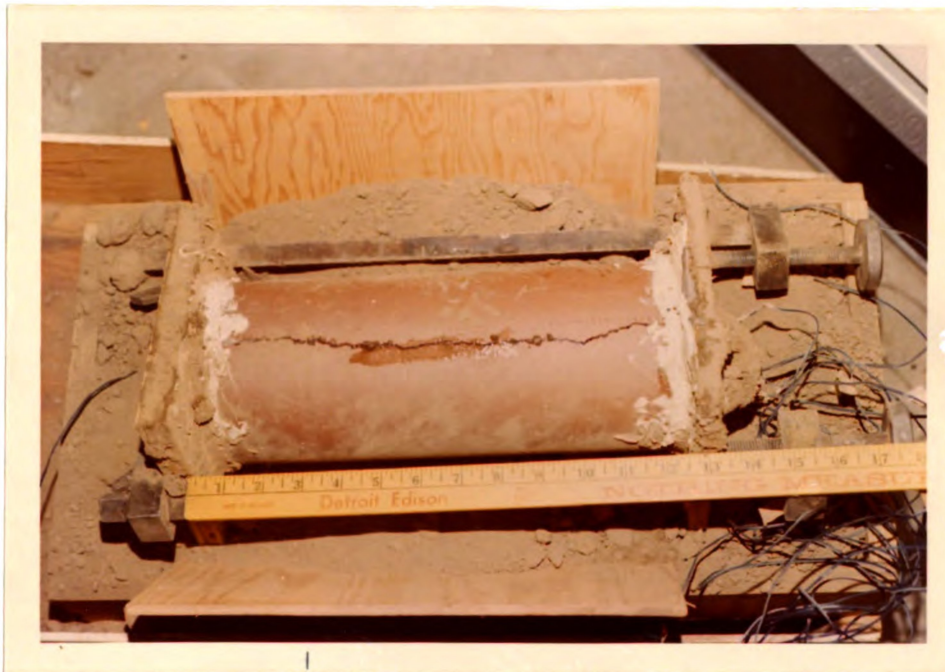
Figure 2-1b. A picture of the cracked tile showing the general appearance. Note the thermocouple wires entering from the right.
