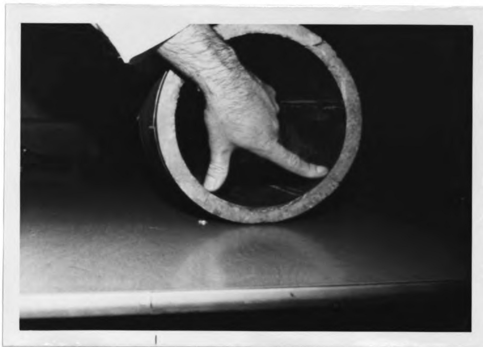
Figure 3-6. A photograph of an 8 inch clay tile removed from a field located near Saginaw, Michigan. Compare the location of cracks with that shown in Figure 2-3.
