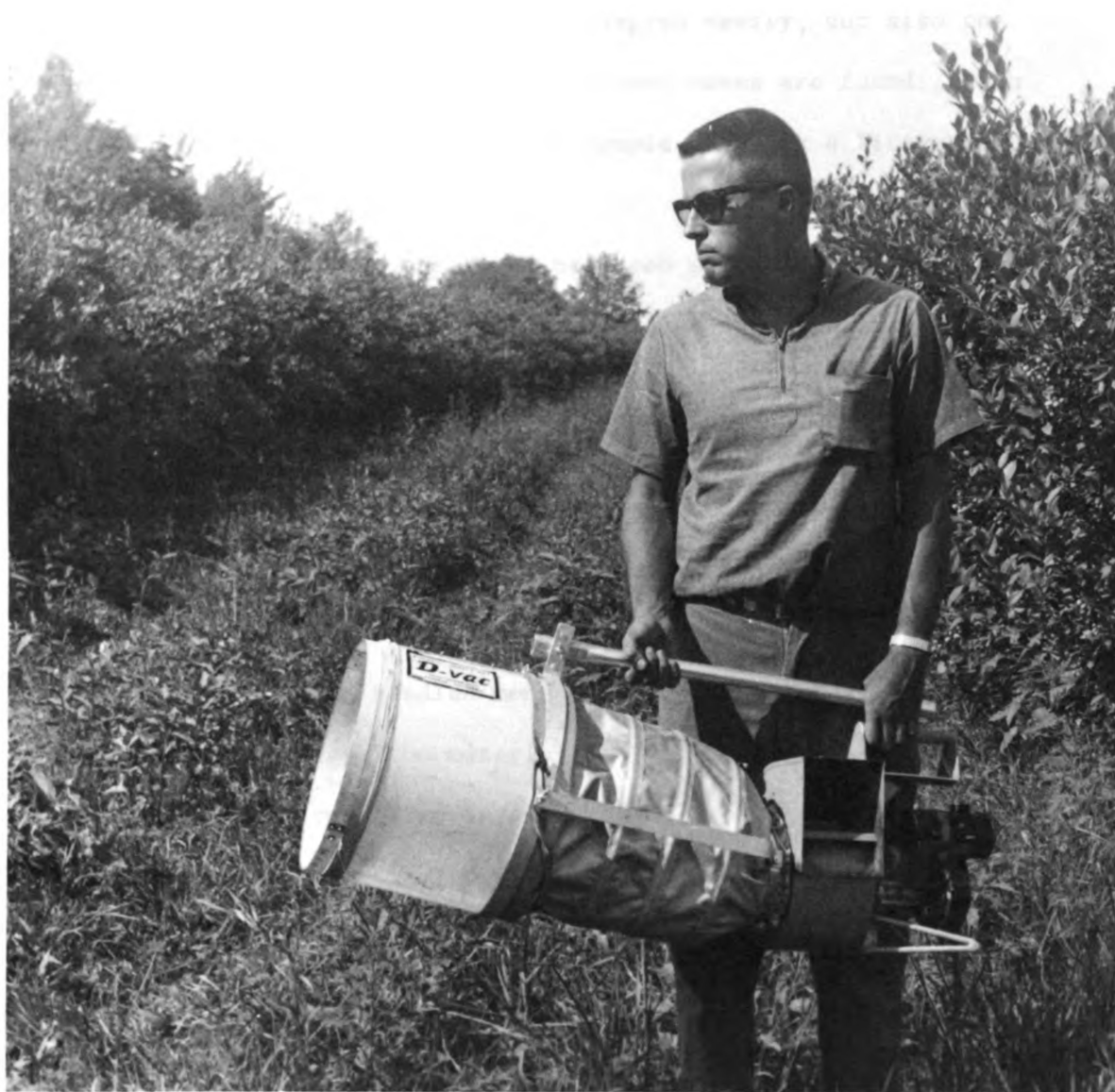
Plate 2.--D-Vac Model 12 Sampler used in survey for collecting taxon found in cultivated blueberry fields.
