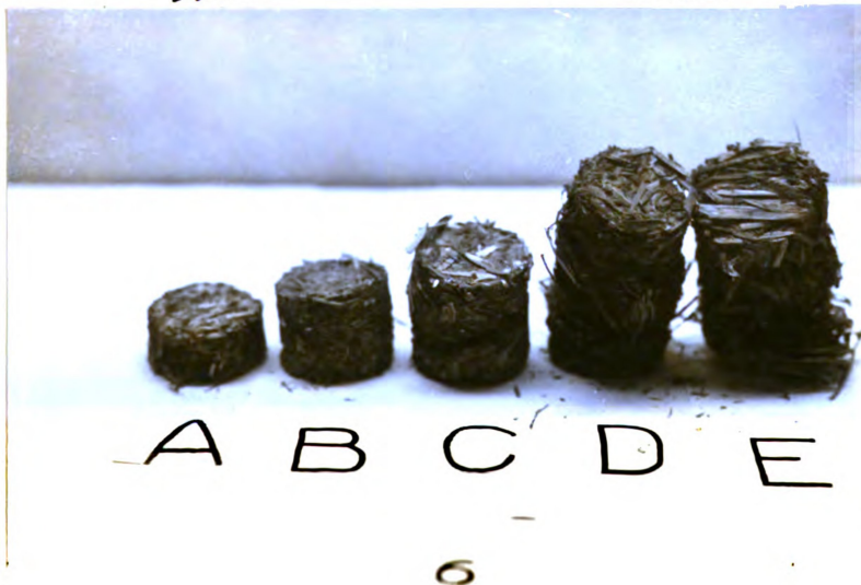
Figure 24. Density-Moisture Relationship with 5000 psi. Pellet Moisture Content-% Density-lbs. per cu. ft. A 8.0 31.1 B 12.5 24.8 C 21.0 18.3 D 32.0 13.3 E 39.0 11.1
