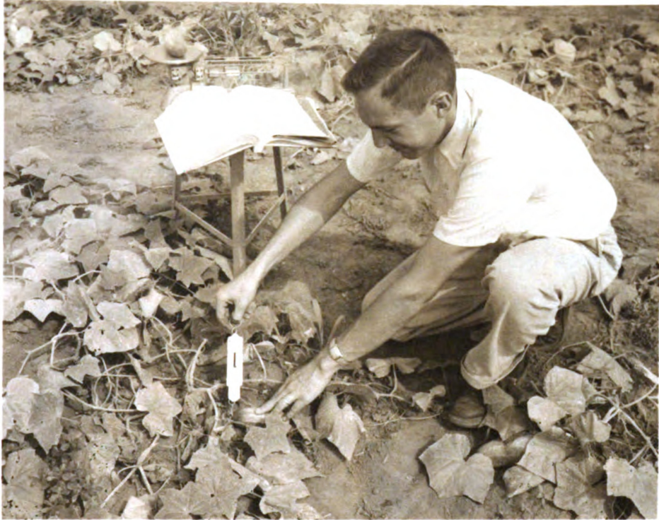
Figure 1. Spring scale used to measure picking force.
