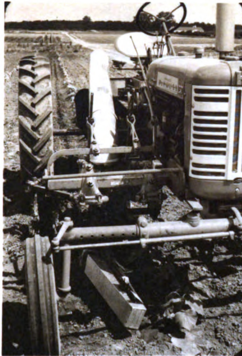
Figure 7. Pneumatic vine trainer mounted on IHC Model 230 tractor.
