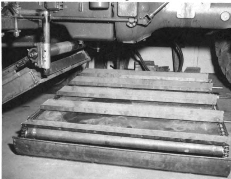
Figure 10. Side view of vacuum pickup unit. Note sheet metal vacuum chamber inside the belt, the transition elbows and the two rollers mounted on the front of the picking bed.
