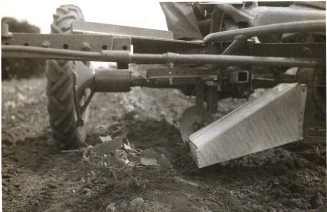
Figure 8. Pneumatic vine trainer in action mounted on Allis-Chalmers Model G tractor.
