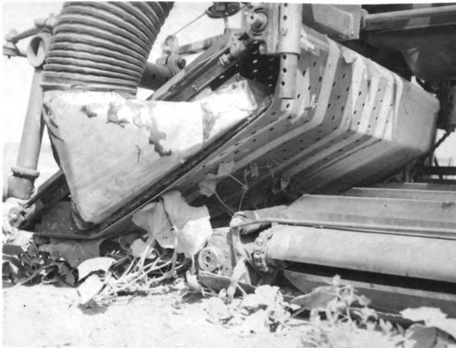
Figure 10. Side view of vacuum pickup unit. Note sheet metal vacuum chamber inside the belt, the transition elbows and the two rollers mounted on the front of the picking bed.
