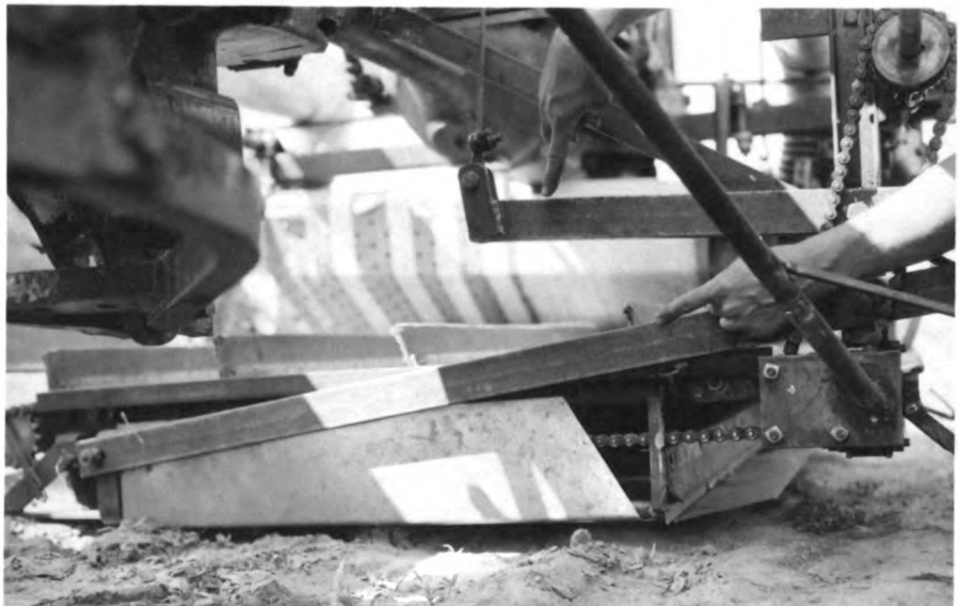
Figure 15. Picking bed lift linkage. Note the picking bed roller chain drive at right.
