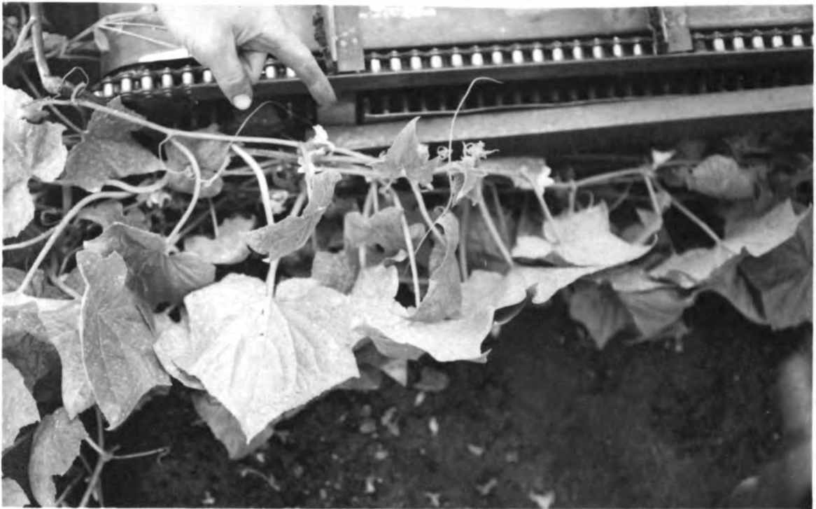
Figure 23. Top view of vines falling off rear of picking bed.
