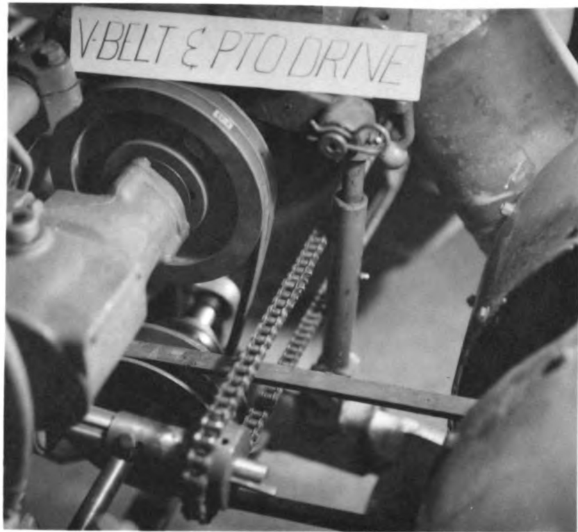
Figure 14. Drive connections to tractor. V-belts power fan and roller chain from PTO drives the machine.
