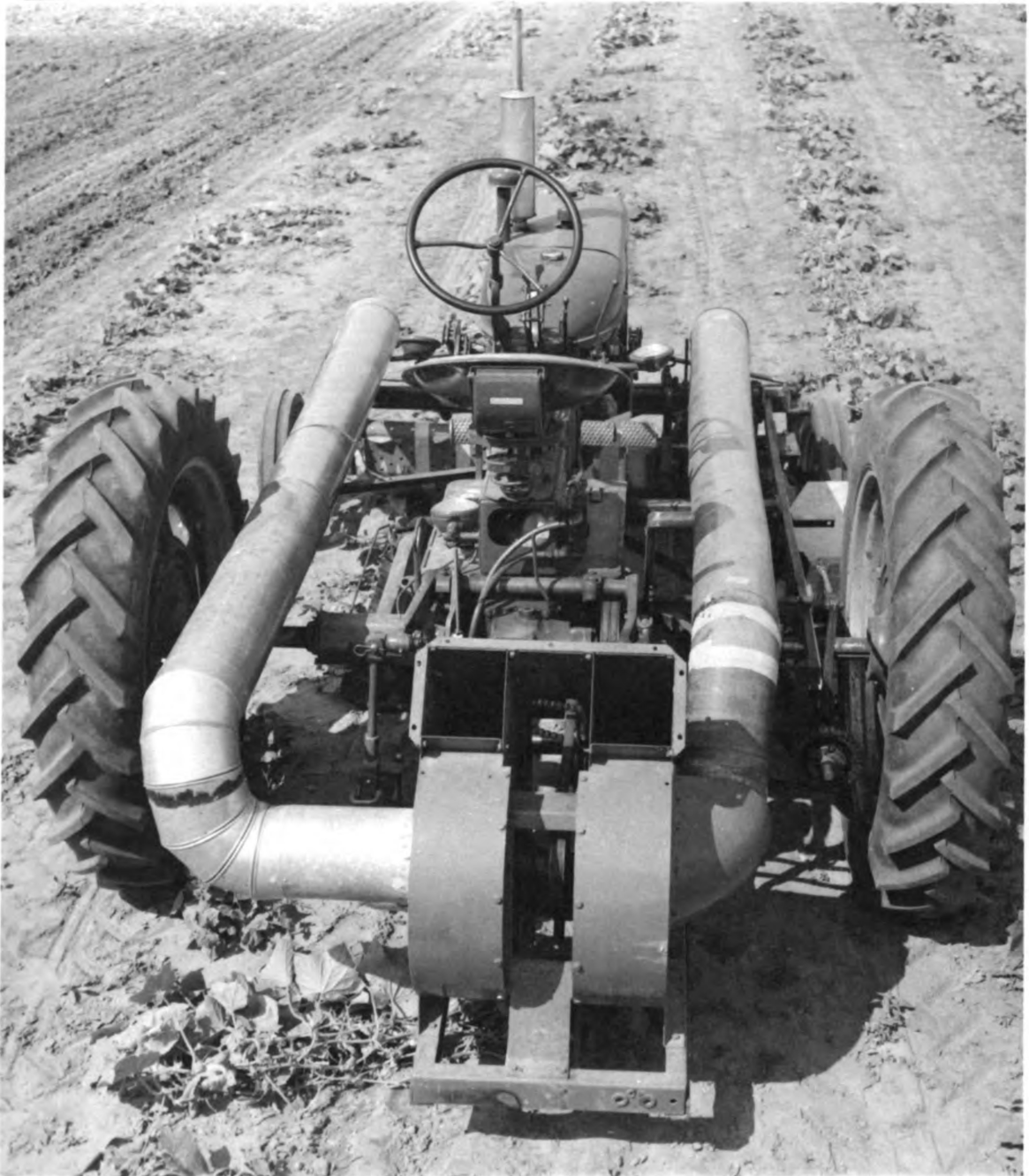
Figure 13. Rear view of harvester showing fan and ducts, main frame along right side and main drive shaft directly under main frame.
