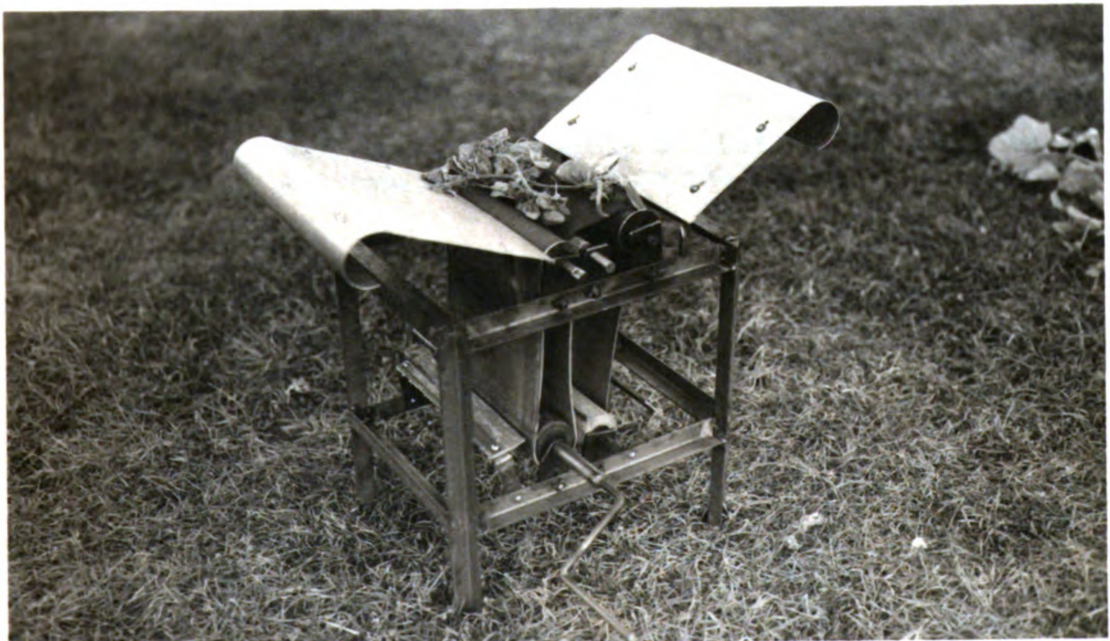
Figure 7. A double belt fruit detachment device with a plant ready for entry into the constriction.
