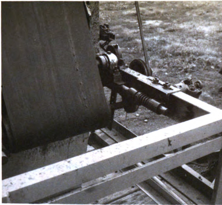
Figure 12. The spring loaded mounting bracket for the spring loaded roller.
