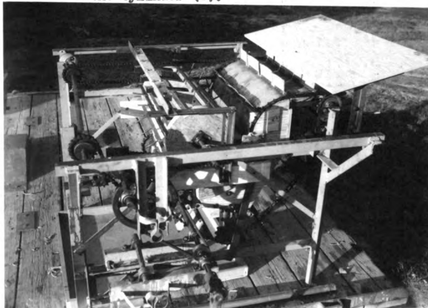
Figure 5. One half of the rotating-cylinder, moving-concave device.
