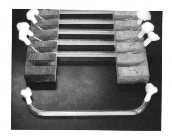
Figure IV Pyrex growth tubes showing their linear shape and method of support.
