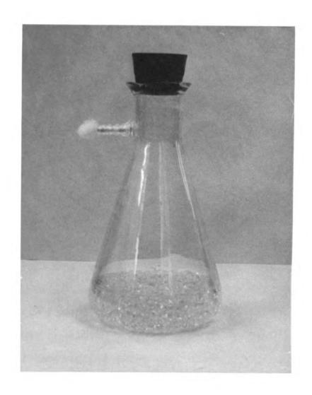
Figure V Shake culture inoculum flask, showing the #6 solid glass beads immersed in the buffer solution.
