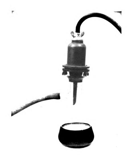
Figure II Seitz filter and suction flask apparatus
