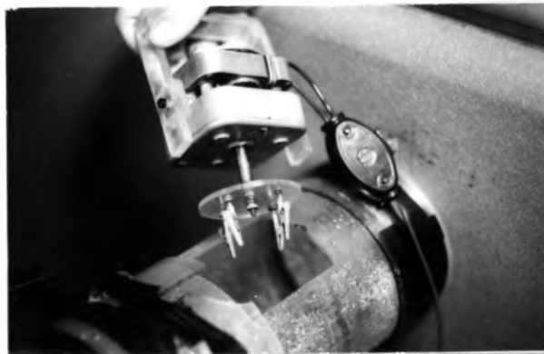
Figure 2.--Revolving platform with clips for holding plant material. View is just above the treatment chamber.
