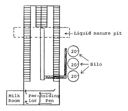
Figure 3. Eighty cow warm-enclosed free-stall barn. Similar plan to Figure 2, except here walls and ceiling are insulated and mechanical ventilation has been installed. Conditions in barn can be controlled regardless of outside conditions.
