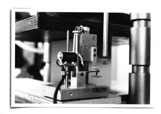
BALDWIN Stress-Strain Recorder (Model MA1B)
