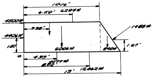
$uexpht = 10.16 \times 4 \times 150 + \frac{2.83}{2} \times 4 \times 150 = 6086 + 849$  = 6.945 # upstream -  $u.p. = wb^{2} = 62.5 \times (14 + \frac{90}{62.5} \times 2)^{2} = 8.906 \#$   $h.s. = 62.5 \times 16.9 \times \frac{3}{4} \times 13 = 4577 \#$
