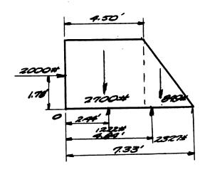
Weight =  $45 \times 1 \times 150 + \frac{2.63}{2} \times 4 \times 150 = 2700 + 619$ Water pressure =  $\frac{10.5}{2} \times \frac{1}{2} \times \frac{1$
