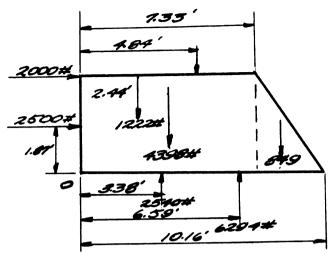
weight =  $73314150 + \frac{2.83}{2}1150 = 1398 + 849$ water pressure =  $\frac{Nh^2}{2} = \frac{625 \times 12}{2} = 4500 #$  1500 - 2000 = 2500 # 1500 - 2000 = 2500 #Center of pressure =  $\frac{16}{12 \times 10} + 10 = 10.13$   $2M_1 = 0$   $23/18 + 4675 - 2540 \times 338 + 23271 \times 841 + 2000 \times 4 + 12221 \times 241 = (5247 - 2500 + 2325 + 1222) \times 1000 \times 1000$
