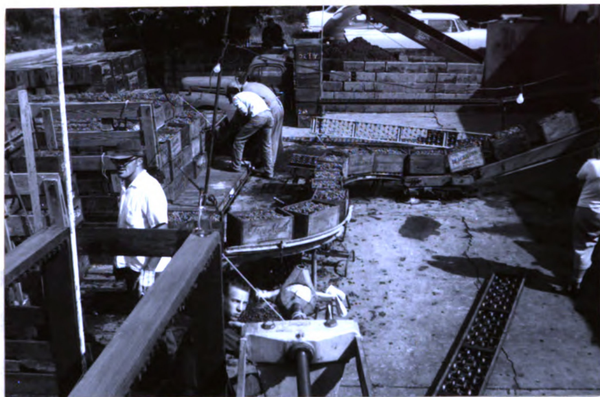
Fig. 17.--Beer lugs of grapes at the Paw Paw Grape Juice Co. processing plant. Arriving by truck transportation, the lugs are carried into the plant on roller conveyors. In the background is a pile of "cheese", or grape pulp left after processing. This is returned to the vineyard where where it is used for fertilizer and erosion control (Paw Paw, Sept. 28, 1959).
