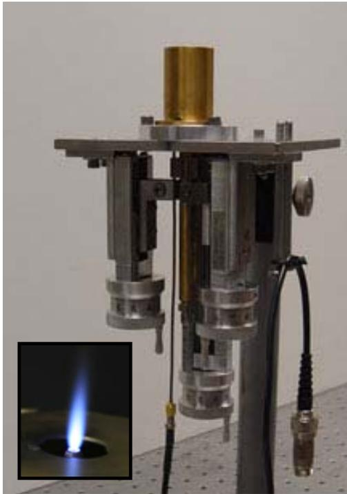
Figure 3.1: Picture of coaxial re-entrant cavity applicator with three fine adjustments using unislides; picture of methane/oxygen flame shown in the inset.
