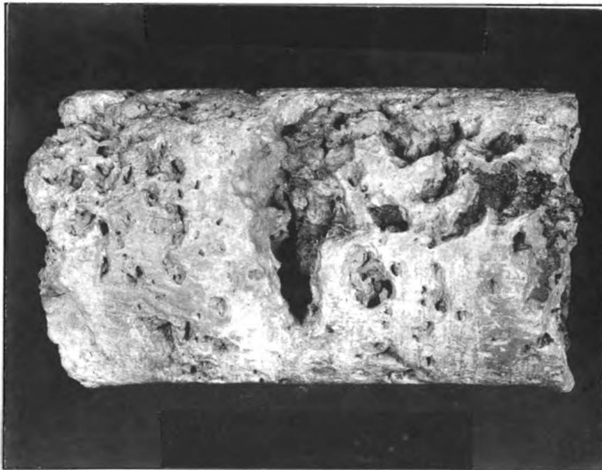
FIGURE 9. DIAMOND-CUT CORE OF "UNIT TWO" FROM GULF NO. 3 MARY PAULSEN AT THE DEPTH OF 1588 FEET SHOWING HIGH [REDACTED] POROSITY.
