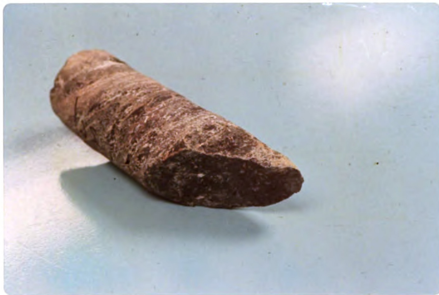
Photo 13: Section of core from the Consumers Power - Brine Disposal #1. Note heavy alteration along broken face and how the angle of break is equal to the foliation
