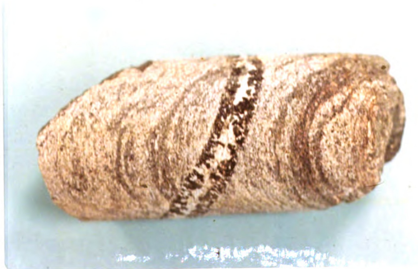
Photo 12: Section of core from the Consumers Power-Brine Disposal #1. Note band of injected material cutting across foliation
