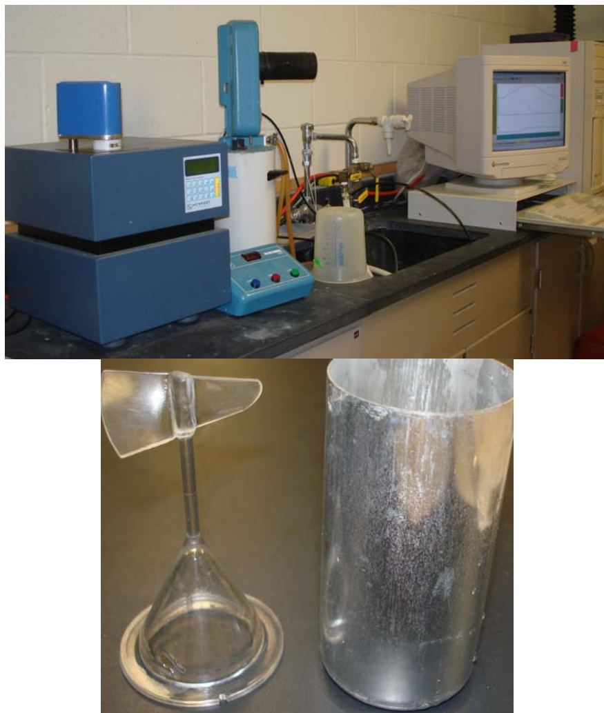
Figure B.2.1. RVA equipment and RVA impeller
