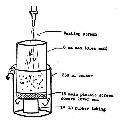
Fig. 1. Washing device for cleaning best seedballs used in the trapping assay for <u>Rhizoctonia</u>.
