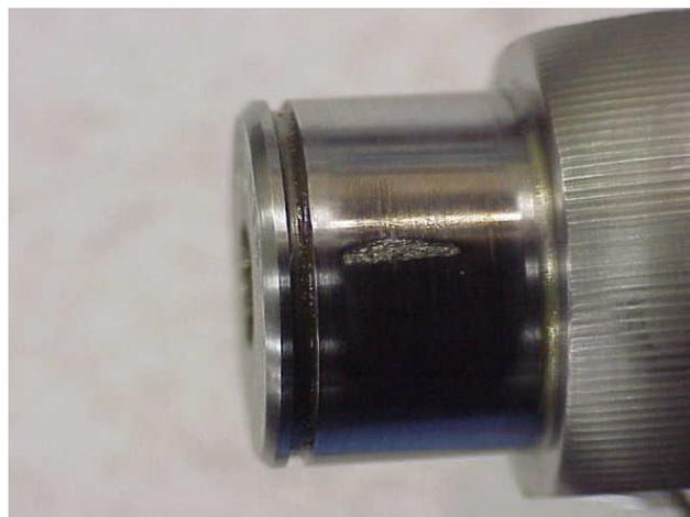
*Figure 4.15. Example of initial wear in a trunnion*
