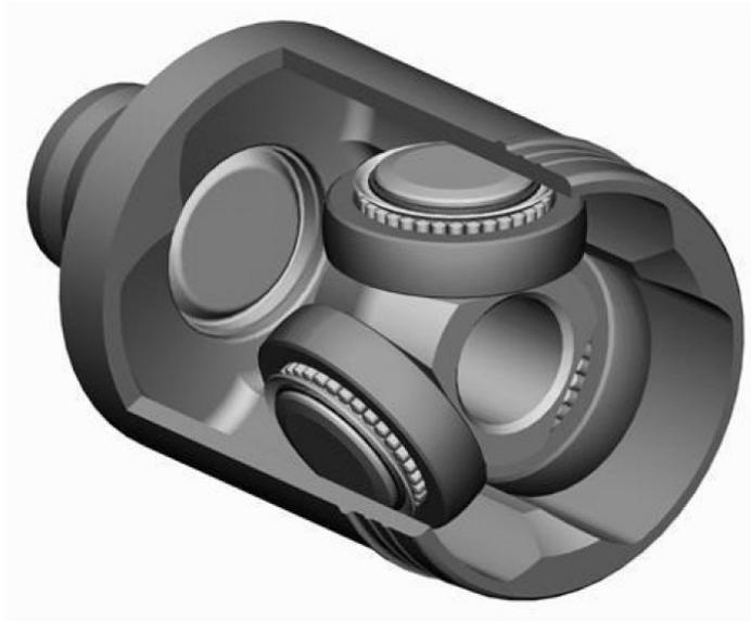
*Figure 1.6. Tripode Joint*
