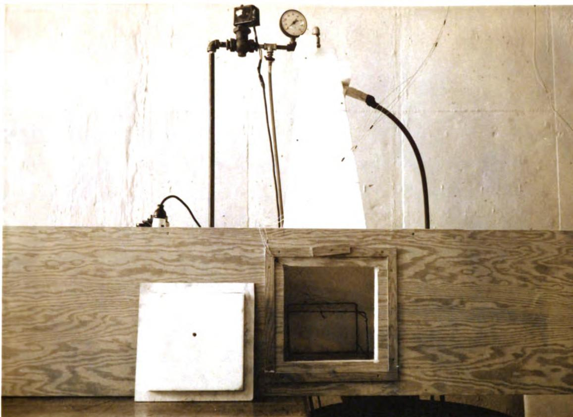
Fig. 5. Close-up showing leaf support, solenoid valve, waste line, pressure gage, spray nozzle, and insulated pyramid.
