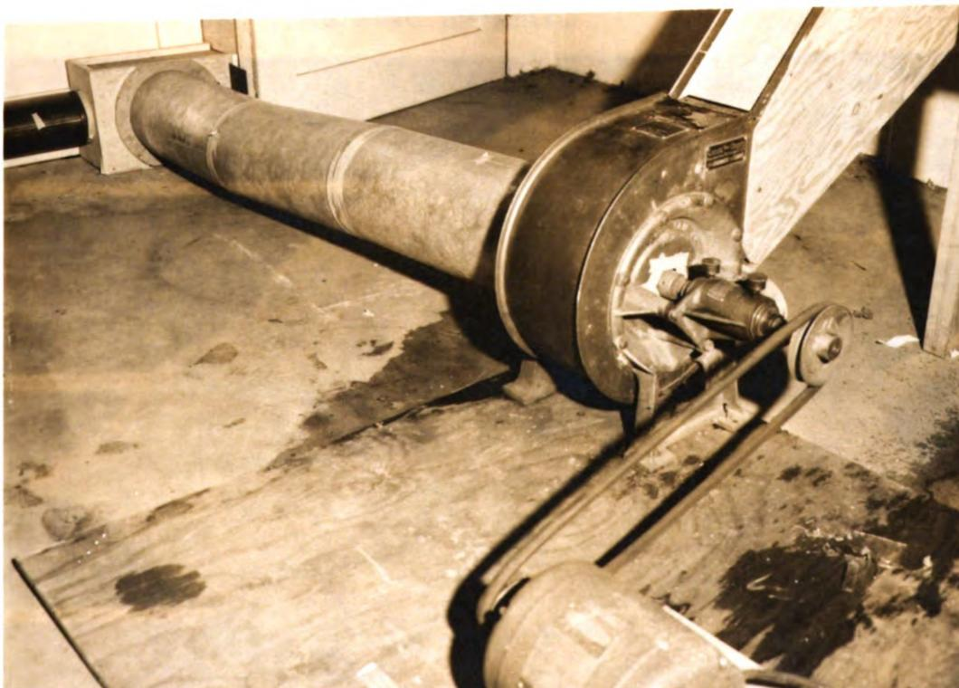
Fig. 4. Close-up showing air temperature mixing box, fan, and conduit to test tunnel, insulation removed.
