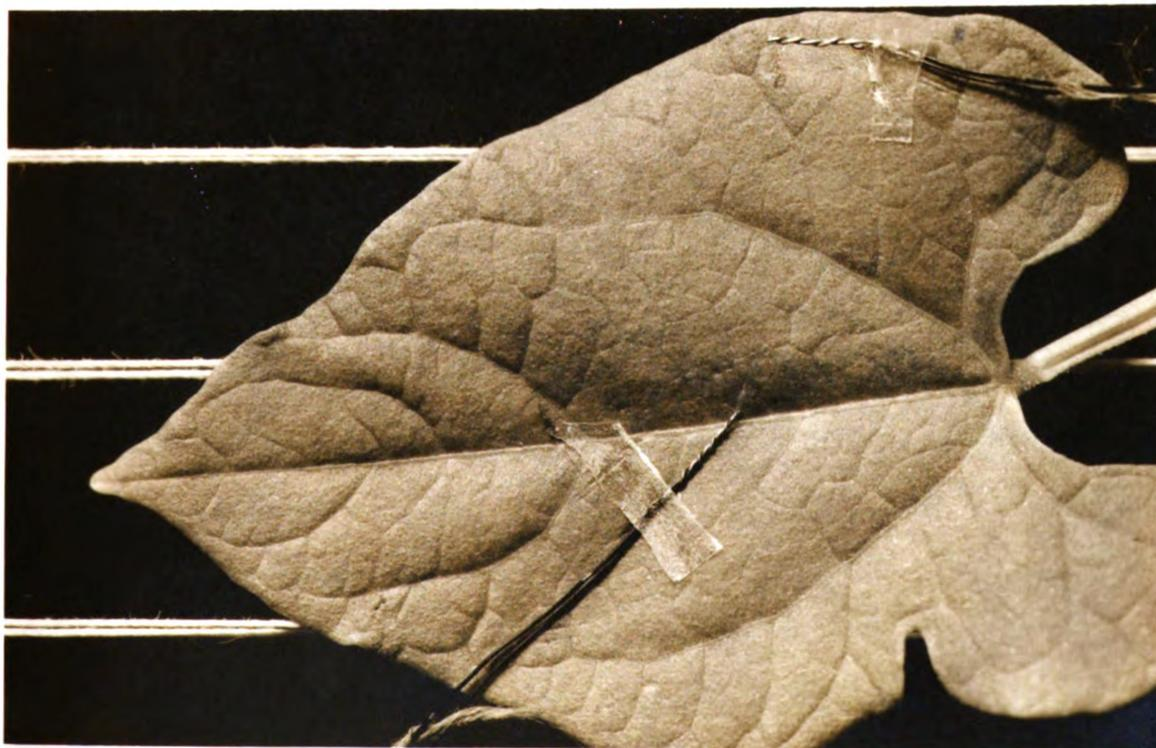
Fig. 6. Thermocouples attached to a leaf.
