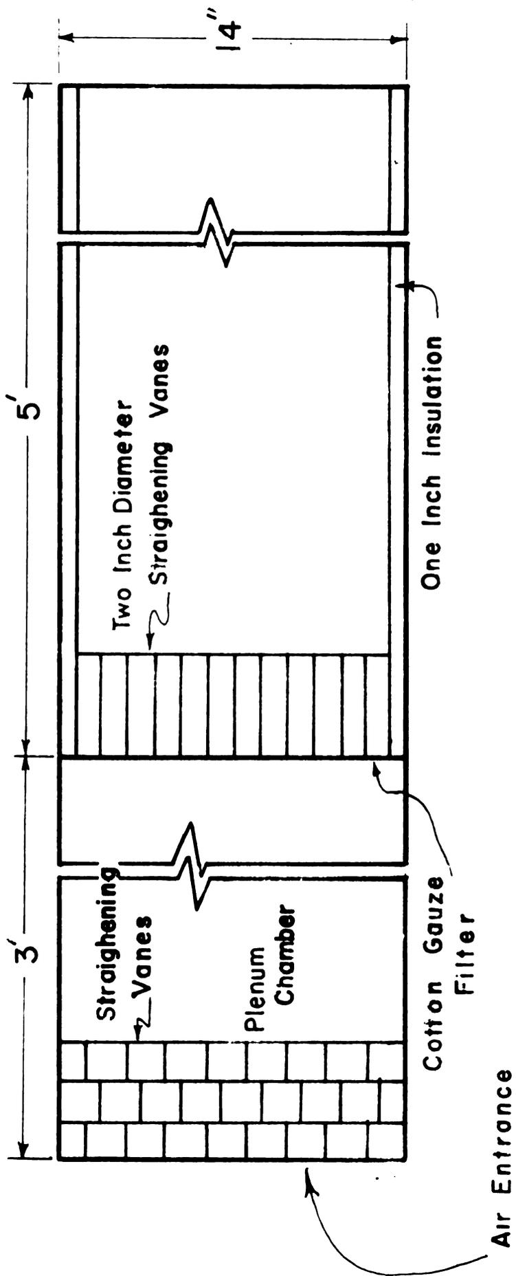
FIG. 2 SCHEMATIC OF TEST TUNNEL
