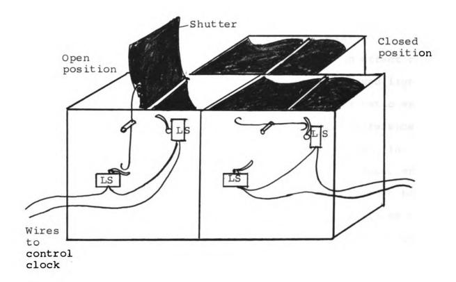
Figure 1. Motor driven Light:Dark boxes. At a time set on the control clock the shutter turns 90 simulating either dawn or dusk. Limiting switches (LS) check the travel of the shutter. Each box is controlled by a separate clock which automatically resets itself.
