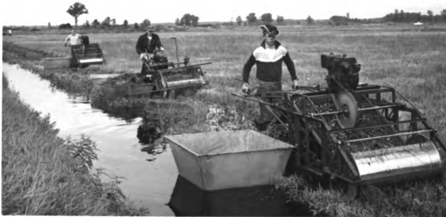
Fig. 32. -- Harvesting by machine. Boat is pulled by machine, lifted on a truck when full. Water must be deep enough to float the boats.
