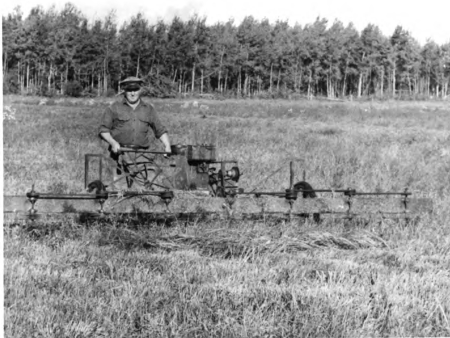
Fig.19. -- A motorized knife clipper in action. Grasses and other weeds growing above the level of the vines can be controlled by this machine. (Northern part of Central region).
