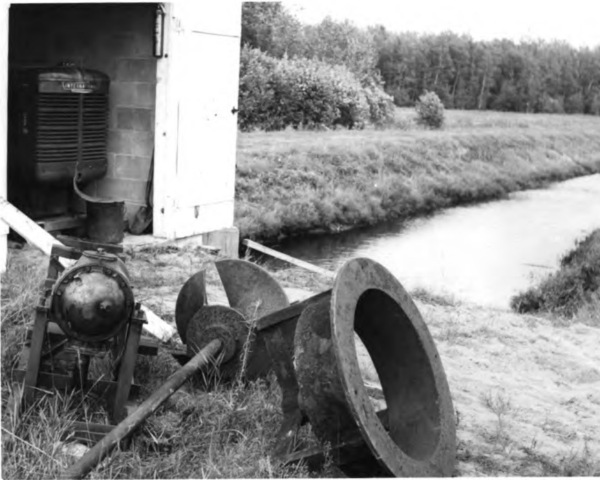
Fig. 14. -- Water pump between reservoir and main canal. These pumps are usually of a screw type as can be seen by the parts in the foreground.
