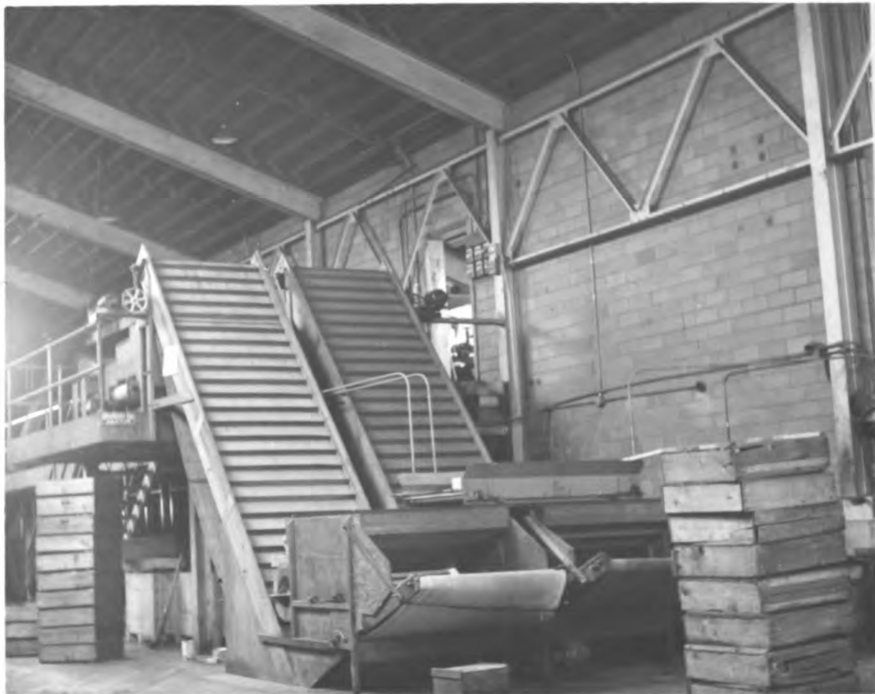
Fig. 35. -- When berries are ready for packaging they are dumped into these conveyors. From here the berries are selected for quality by a machine and then by hand. Cranberries are now packaged mostly in cellophane bags.
