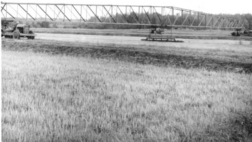
Fig. 21. -- The latest in cranberry marsh mechanization, the "bridge." Trucks on each end move forward as carriage moves back and forth, clipping or spraying. Need for beds of uniform size and levelness is obvious for a modern marsh.
