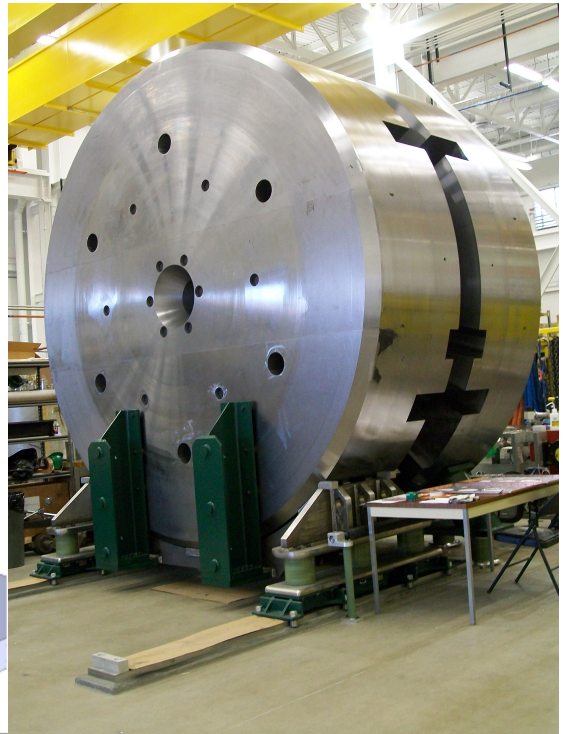
Figure 7.5: Left: Schematic of the cyclotron gas cell. Right: The cyclotron magnet yoke as of April 2013.
