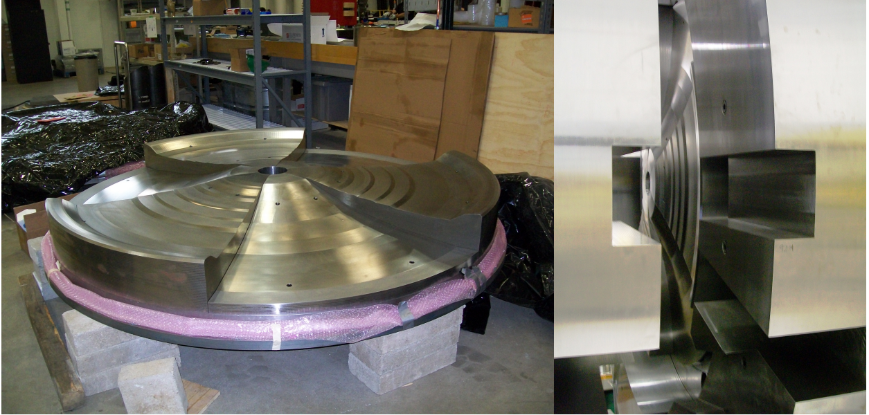
Figure 7.1: Left: Photograph of the six sector magnet pole steel during assembly. Right: Photograph of the pole steel inside the vertical magnet yoke of the cyclotron gas stopper.
