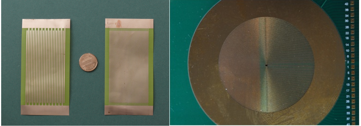
Figure 2.3: Examples of the two RF carpet electrode geometries. Left: RF carpets with linear electrodes (and two different pitches) used by Pang [10]. The pitch, a , is the sum of one electrode and one gap width. Right: RF carpet with concentric electrodes developed and employed by Wada [3].
