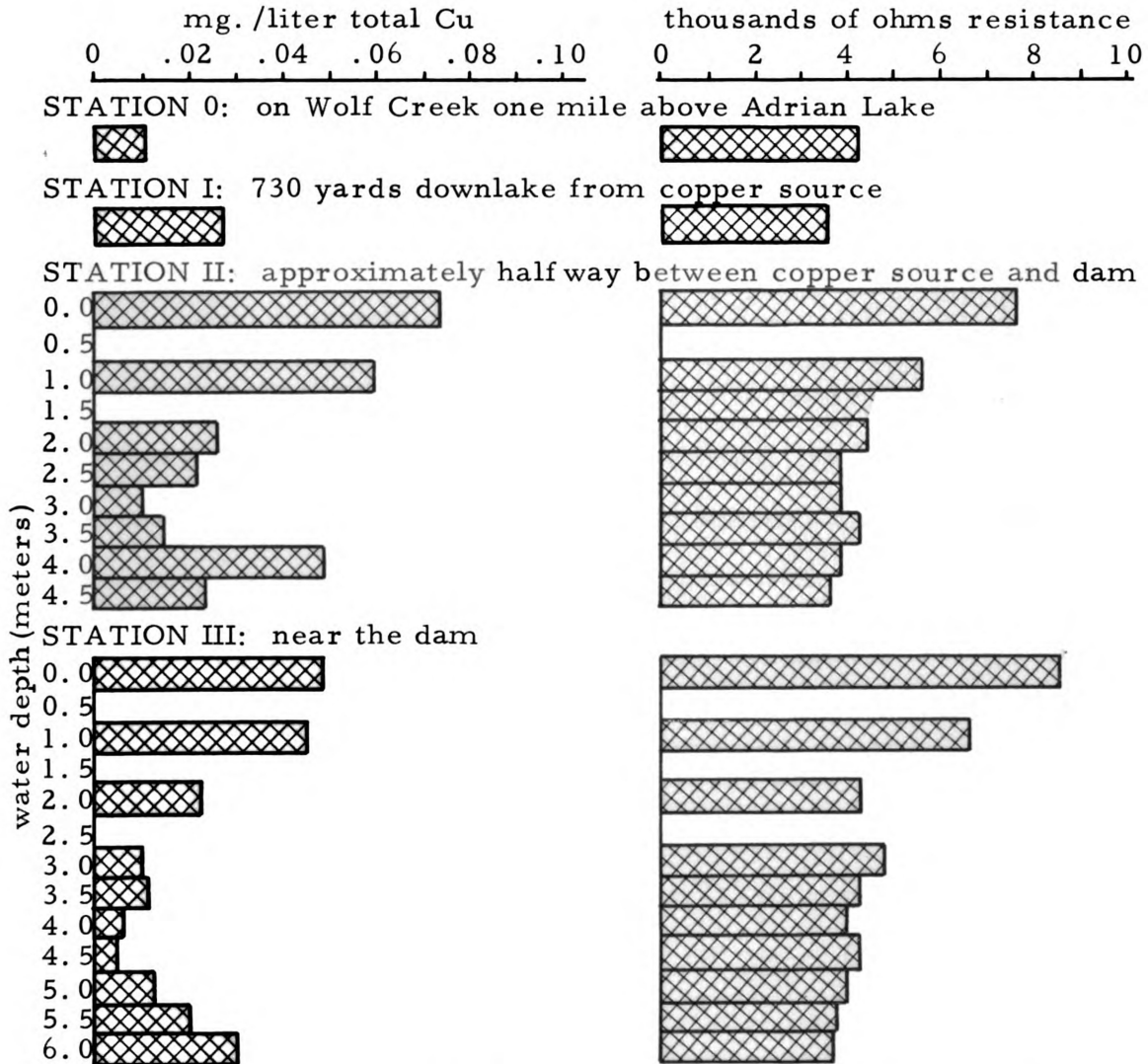
Figure 5. Comparison of total copper concentration and lake water resistance data for March 15, 1965, which illustrates the effect of a density current on copper concentration. The \text{CuSO}_4 feed device was shut down an entire month prior to this date.
