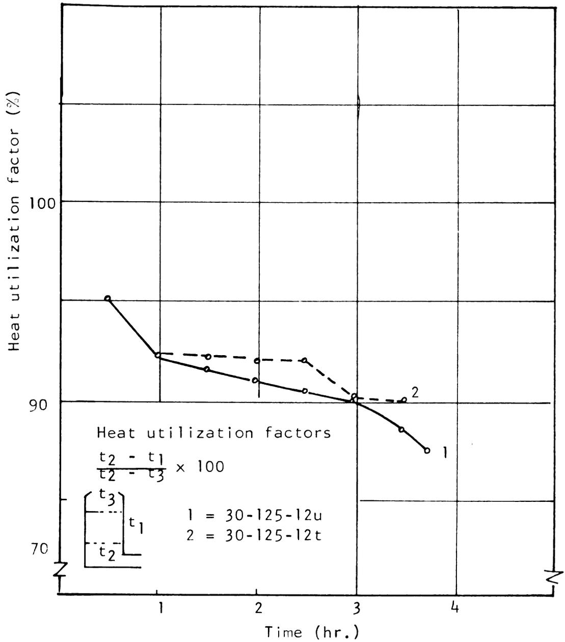
Figure 22. The effect of periodic tempering at 125°F drying air temperature on the heat utilization factor
