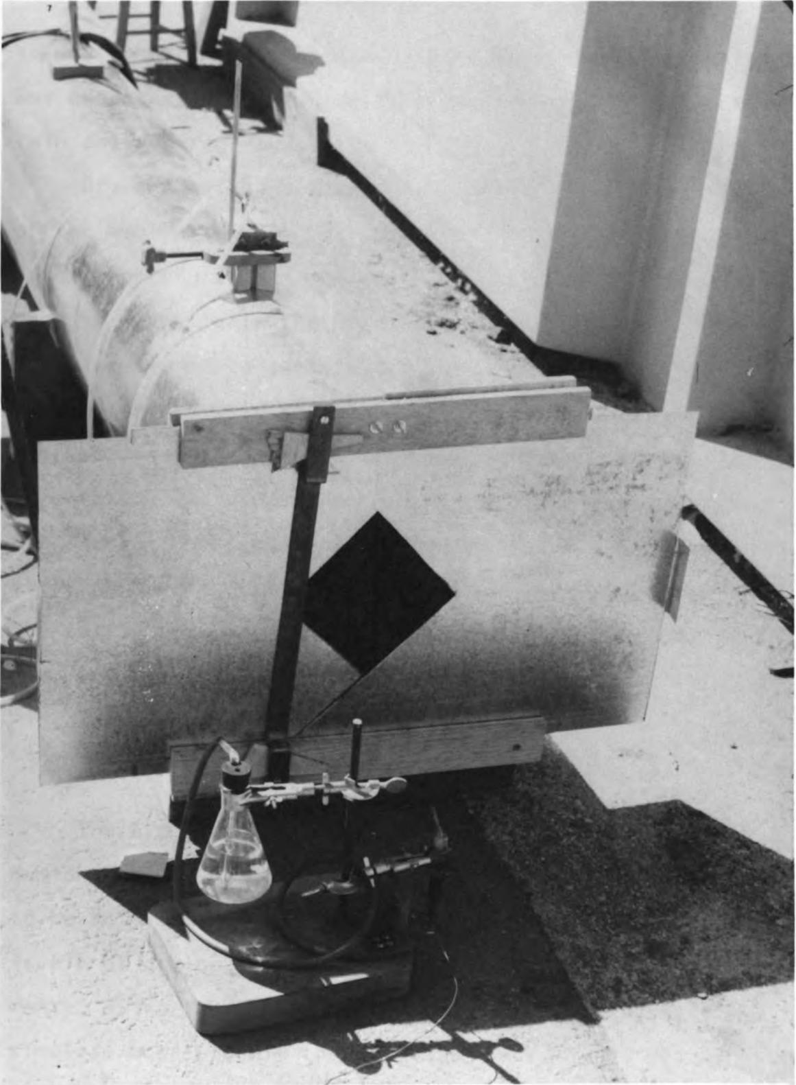
Figure 4. Wet-bulb temperature measurement and the sliding gate at the outlet of the measuring tube. By opening and closing the sliding gate the static pressure was varied.
