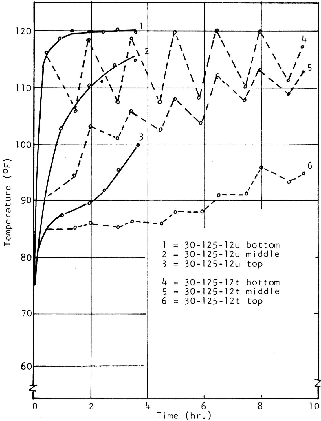
Figure 21. The effect of periodic tempering at 125°F drying air on grain temperatures
