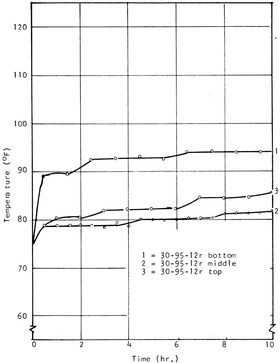
Figure 19. The effect of periodic air flow reversal at 95°F drying air temperature on the grain temperatures
