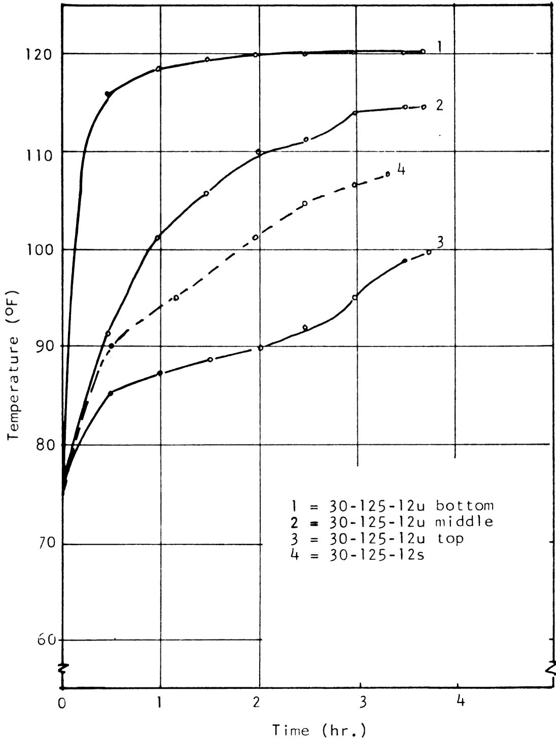
Figure 15. The effect of stirring at 125°F drying air temperature and 12 inch depth on the grain temperatures
