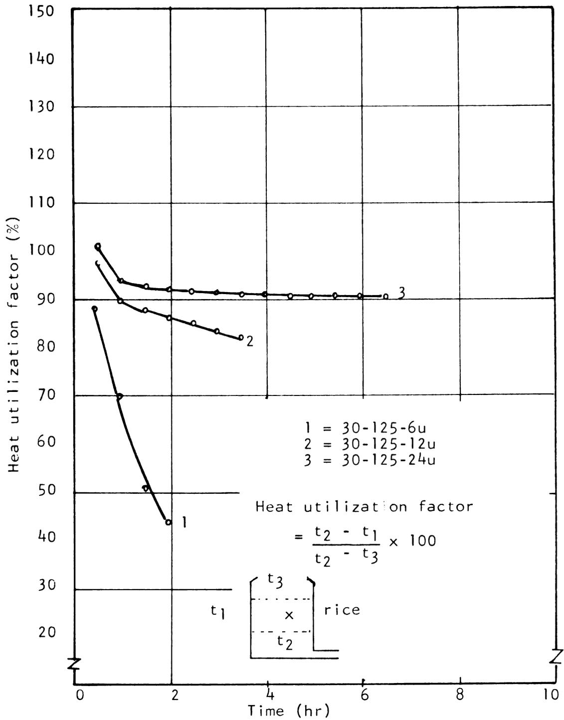
Figure 11. The effect of grain depths on heat utilization factor at 125°F.
