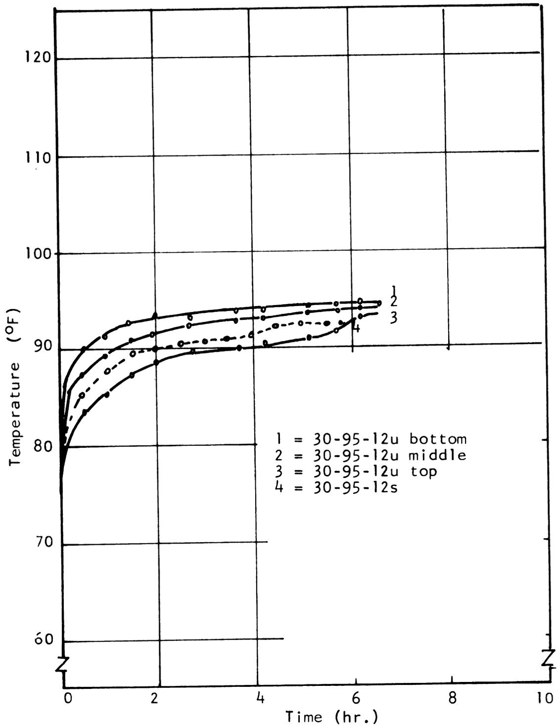
Figure 16. The effect of stirring at 95°F drying air temperature on the grain temperatures.
