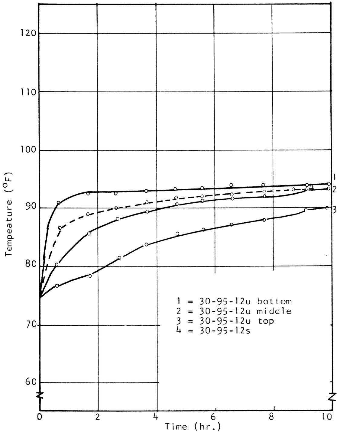
Figure 18. The effect of stirring at 95°F drying air temperature on grain temperatures (stirring for every one hour)
