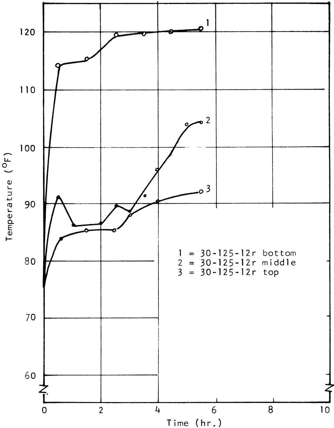
Figure 20. The effect of periodic air flow reversal at 125°F drying air on the grain temperatures.
