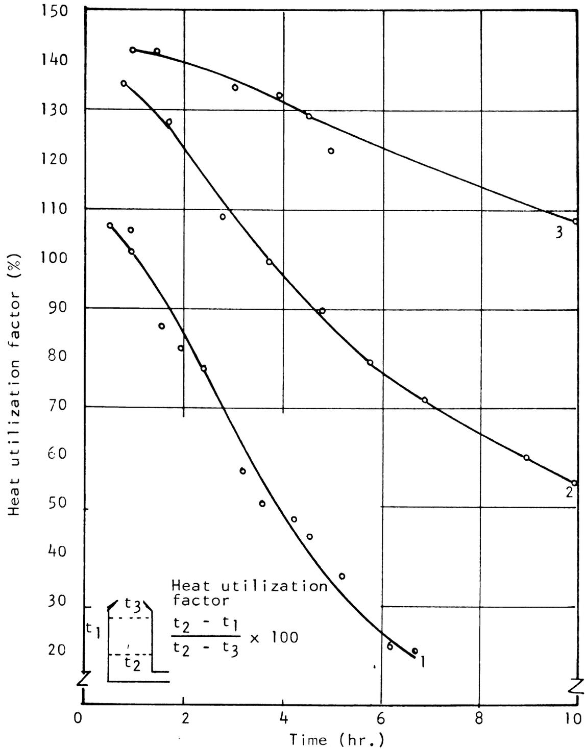
Figure 12. The effect of grain depths on the heat utilization factor at 95°F.
