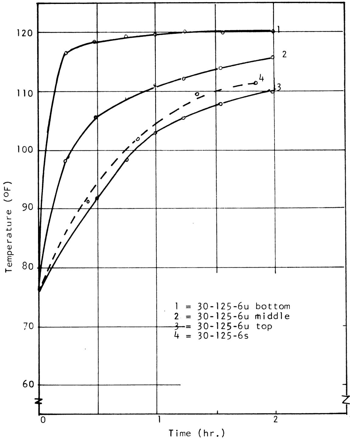
Figure 17. The effect of stirring at 125°F drying air temperature and 6 inch depth on the grain temperature
