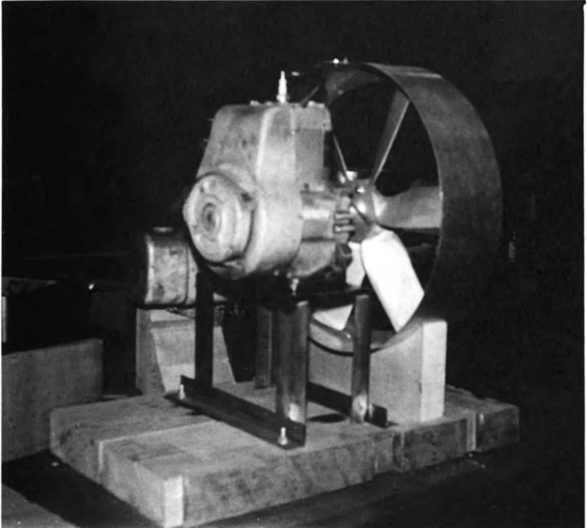
Figure 3. Direct connection propeller fan to the Clinton engine. A tube and plate ring were placed around the propeller housing to direct the airflow and reduce the turbulence of airflow.
