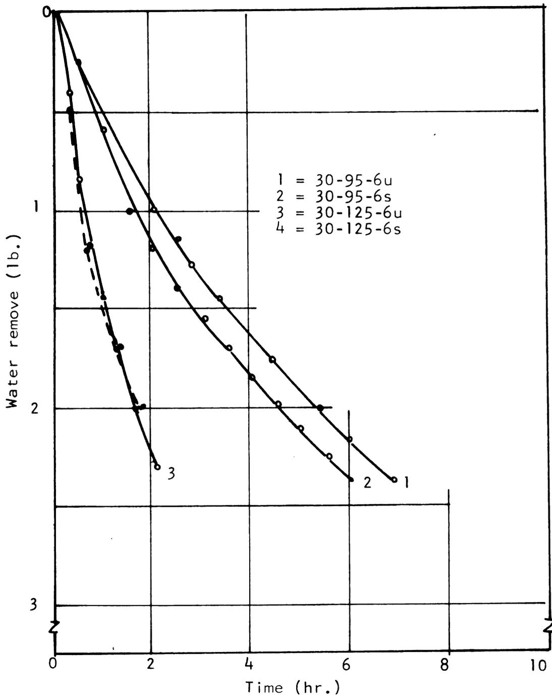
Figure 14. The effect of stirring on the drying rate of rice at the 6 inch depth.
