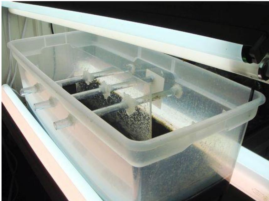
Figure 2: Semi-continuously fed and harvested raceway pond, the culture was circulated using an aquarium pump and exposed under fluorescent lamps.
