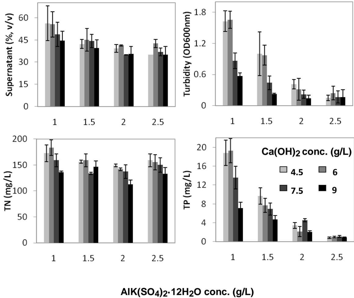
Figure 6: Chemically pretreated AD effluent.  $\text{Ca}(\text{OH})_2$  (4.5, 6, 7.5, 9 g/L) and  $\text{AlK}(\text{SO}_4)_2 \cdot 12\text{H}_2\text{O}$  (1, 1.5, 2, 2.5 g/L) were used as coagulants in the pretreatments. The combination with 7.5 g/L  $\text{Ca}(\text{OH})_2$  and 1 g/L  $\text{AlK}(\text{SO}_4)_2 \cdot 12\text{H}_2\text{O}$  (dashed rectangle) was selected as the optimal pretreatment method, judging by the turbidity, volume, TN and TP of the supernatant.
