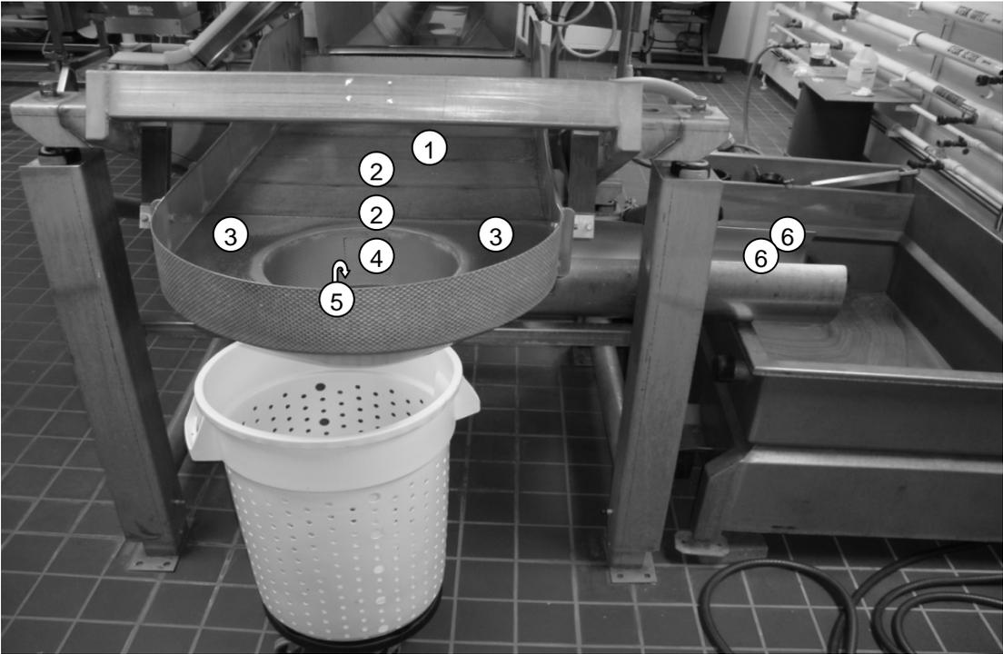
Figure 2.5: *Dewatering centrifuge sampling locations*
