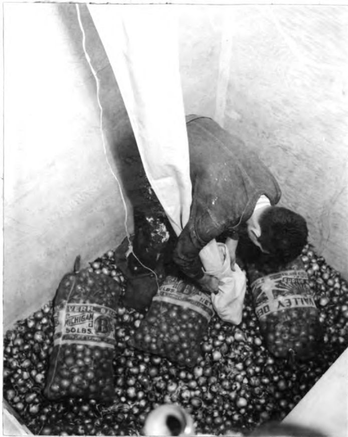
Fig. 13. Showing Placement of Onions in Bin Using Canvass Filling Tube. Also, Note Position of Shrinkage Samples and Thermocouple Wires.
