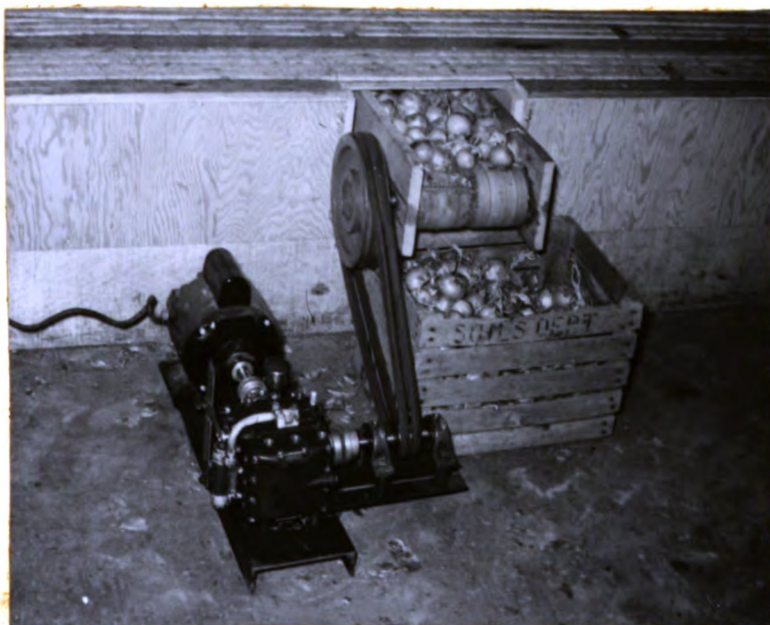
Fig. 19. Driven End of Conveyor with Hydraulic Reduction Unit.
