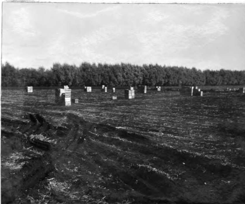
Fig. 16. Field Stacked Shrinkage Sample Crates Showing Conventional Curing Method.
