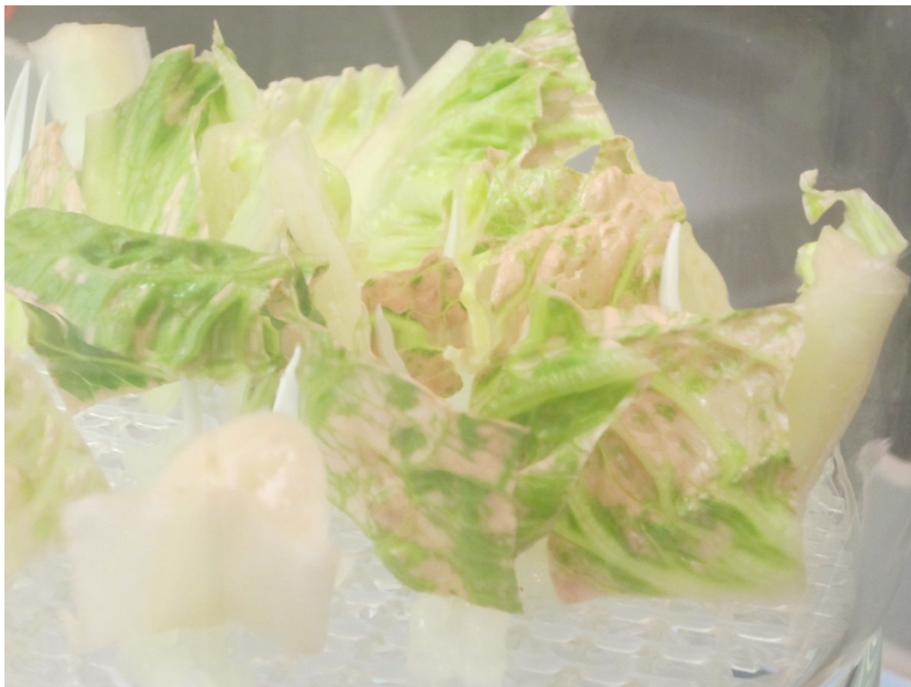
Figure 4.4 - Bleached lettuce after treatment with 6 mg/L for 10 min with the \text{ClO}_2 produced by the Minidox
