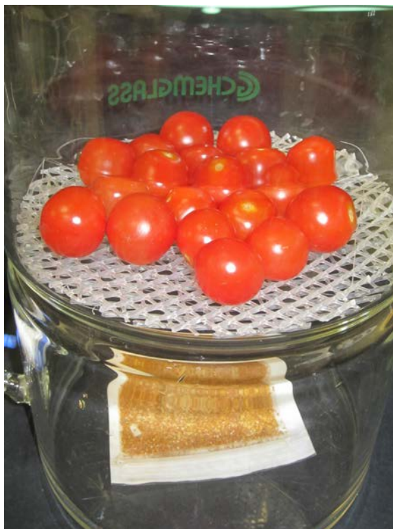
Figure 3.3 - Tomatoes placed inside the glass chamber being treated with \text{ClO}_2 generated by the sachet
