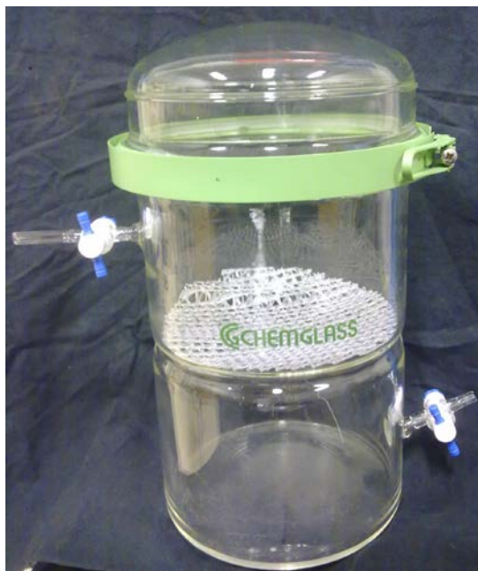
Figure 3.1- Glass chamber for absorption study
