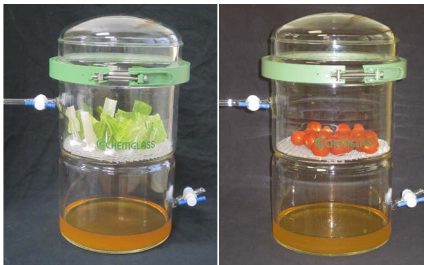
Figure 3.4 - Lettuce and Tomatoes exposed with ClO 2 gas generated by a ClO 2 solution
