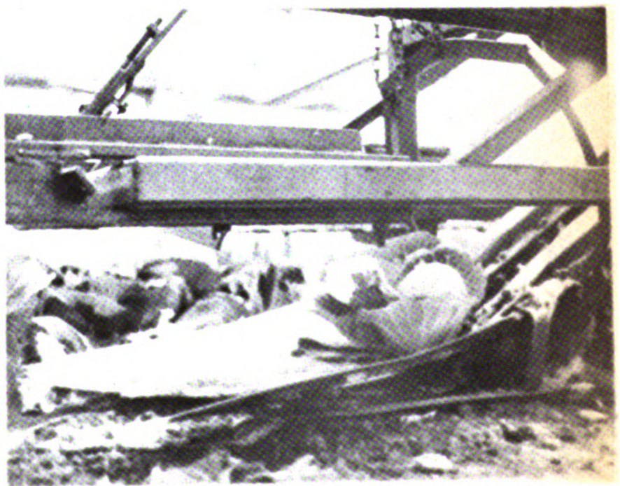
Fig. 8. Lifter shoes of test (7) showing slides and curved shields.
