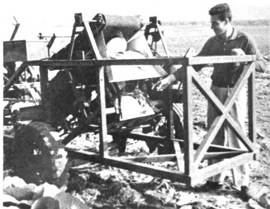
Fig. 24. The paddle wheel mechanism in operation.
