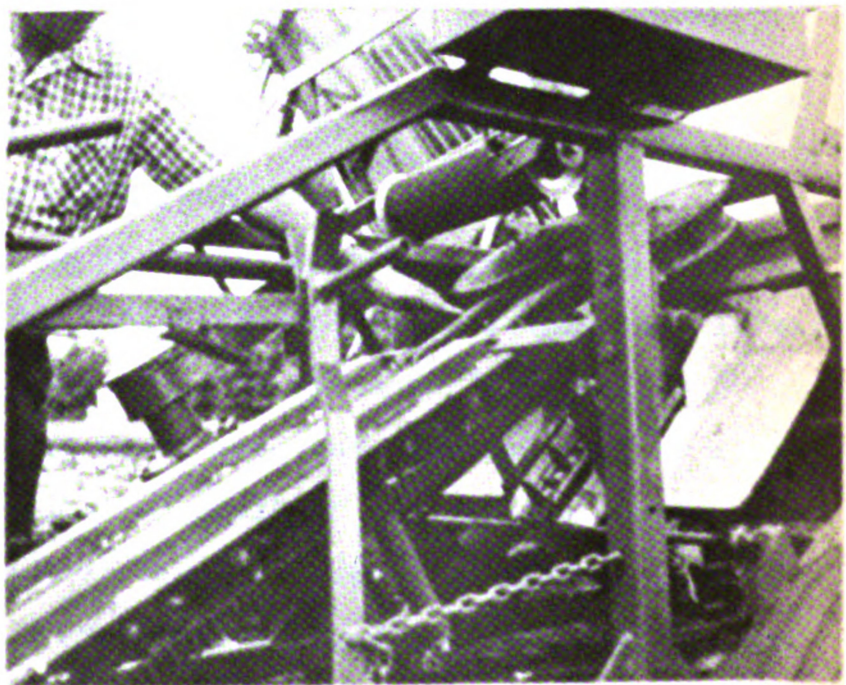
Fig. 4. MSU experimental harvester showing internal roller and roller drive, overhead belt and roller drive.
