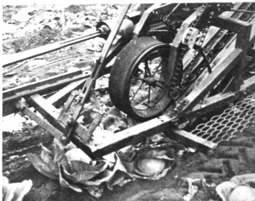
Fig. 16. Floating rubber tire to help lift the cabbage (test 250).
