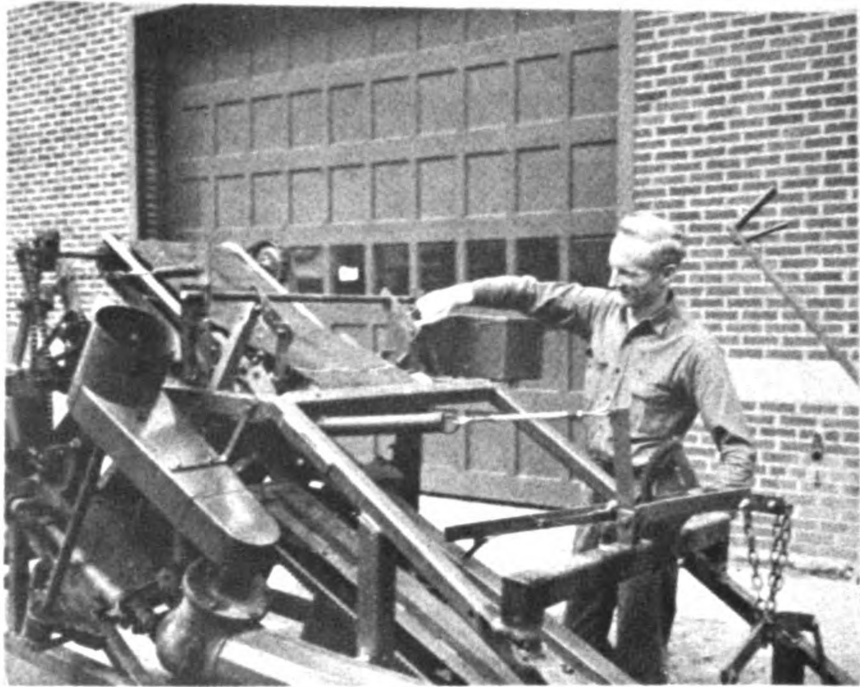
Fig. 27. Spring-loaded suspension of the overhead belt, allowing wider swinging.
