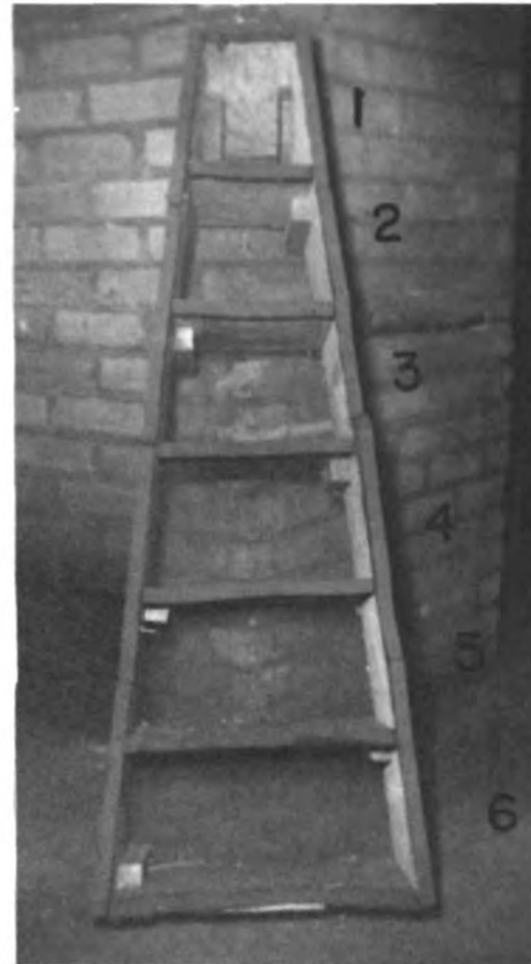
Fig. 7. Sampler box showing equally long sections 1-6.
