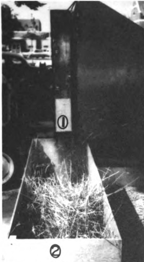
Fig. 6. Material emerging from the straw outlet (1) being collected in container (2).
