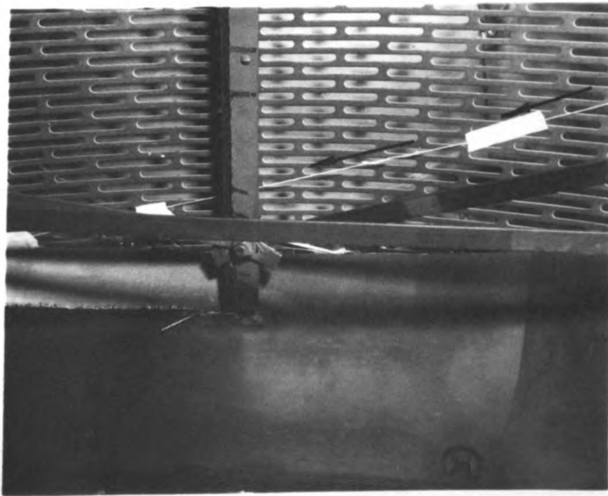
Fig. 21. Direction of the path of a piece of chalk which was fed into the empty cone and made a mark as it passed through.
