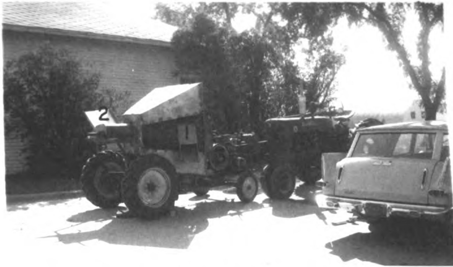
Fig. 9. General view of equipment; (1) circle-sample chute, (2) feeding mechanism, and (3) pulley, belt driven by the tractor.
