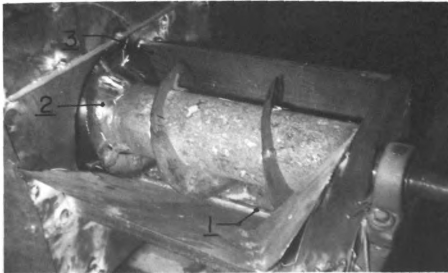
Fig. 8. View of feed-auger showing: (1) steel strip, (2) conical part of auger, and (3) inner surface of the screen.
