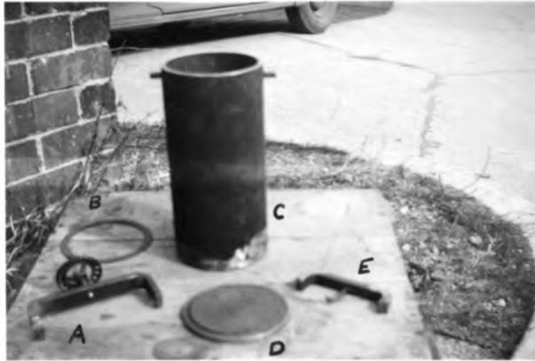
The apparatus for determining the air content of concrete is shown disassembled above.
