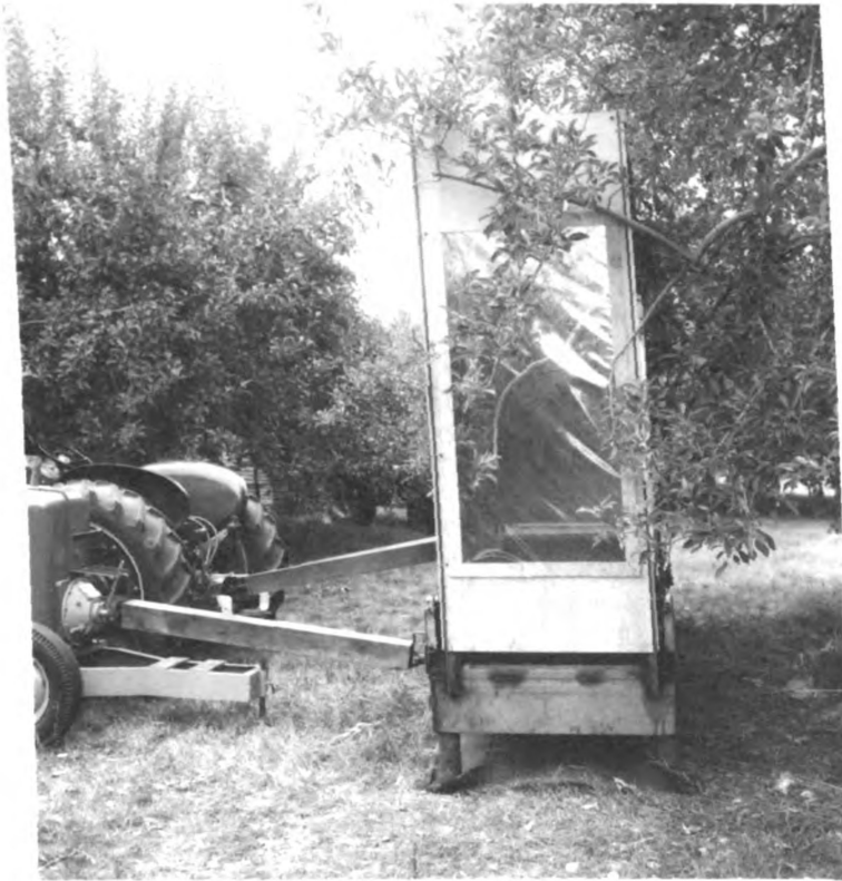
Figure 26. Pneumatic fruit harvester with a limb inside the confining walls.
