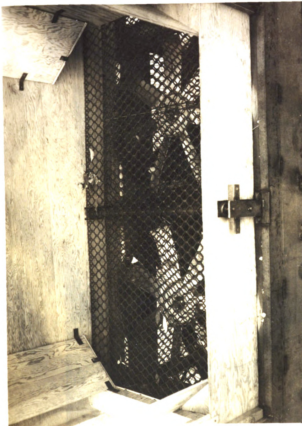
Figure 25. Position of fans beneath the fruit catching and conveyor belt.
