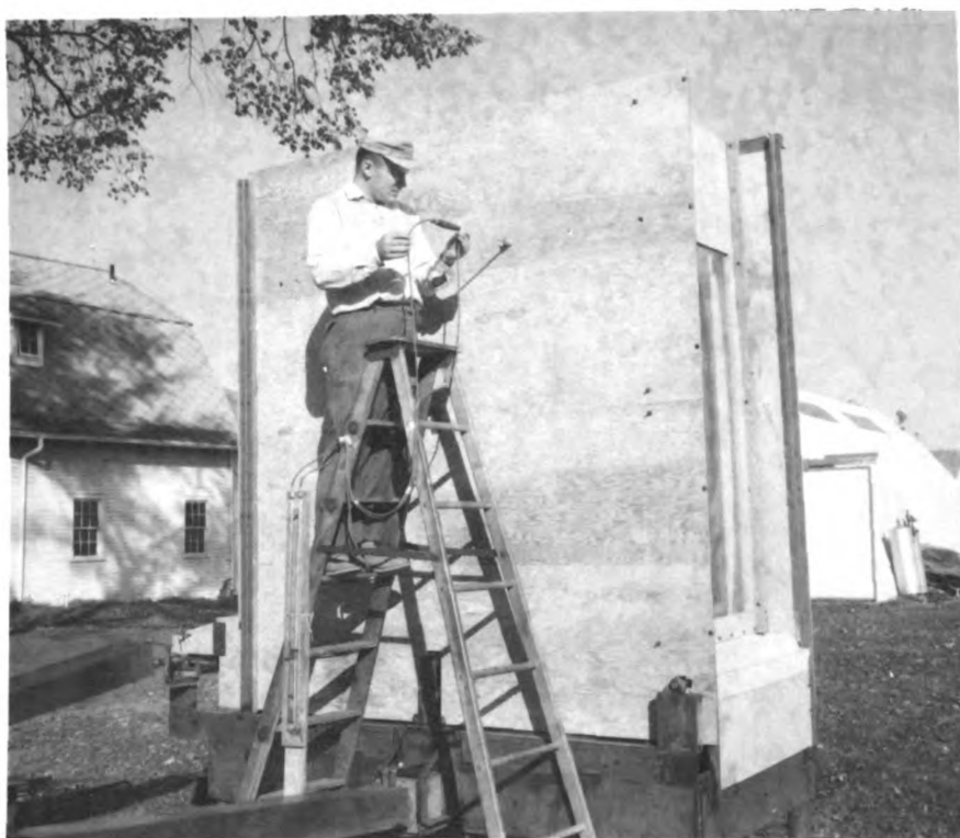
Figure 29. Measurement of air velocity inside the walls with a pitot tube.
