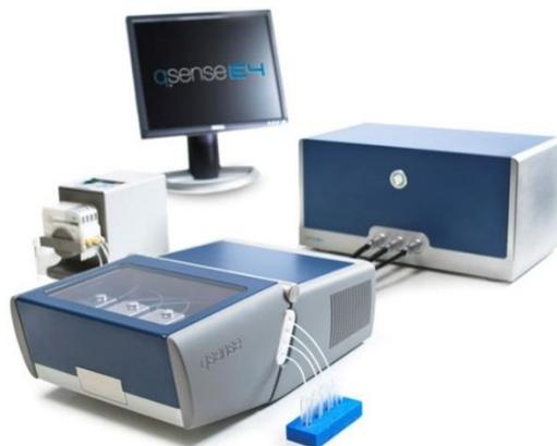
**Figure 2:** QCM-D system (source: q-sense.com)
